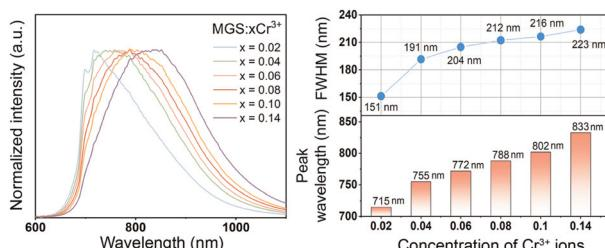
**Achieving tunable ultra-broadband NIR emission originating from the two-site occupation of Cr<sup>3+</sup> ions in  $\text{Mg}_3\text{Ga}_2\text{SnO}_6:\text{Cr}^{3+}$**
