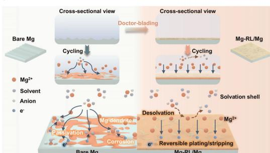
**Mg-Rich LAPONITE® interface protective layer enables reversible, corrosion-resistant anodes for high-performance magnesium metal batteries**
