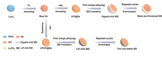
**Regulation of solid–electrolyte interphase formation via a  $\text{Li}_3\text{PO}_4$  artificial layer for ultra-stable germanium anodes**
