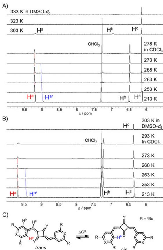
**Fig. 5** (A) VT-<sup>1</sup>H NMR spectra of **SQ2a** in DMSO-*d*<sub>6</sub> (333–303 K) and CDCl<sub>3</sub> (278–213 K). (B) VT-<sup>1</sup>H NMR spectra of **SQ2b** in DMSO-*d*<sub>6</sub> (303 K) and CDCl<sub>3</sub> (293–213 K). (C) Schematic diagram of the thermal *cis*-*trans* isomerization and the Gibbs free energies of activation ( $\Delta G^\ddagger$ ) for the isomerization.
