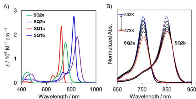
**Fig. 6** (A) The electronic absorption spectra of **SQ2a** (green), **SQ2b** (purple), **SQ1a** (red) and **SQ1b** (blue) in DMSO (5 μM). (B) Normalized electronic absorption spectra of **SQ2a** and **SQ2b** in the temperature range from 373 to 303 K.
