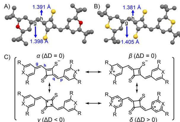
**Fig. 3** Single crystal X-ray structures of **SQ2a** (A) and **SQ2b** (B) at 100 K. Bond lengths of the methine part ( $g$  and  $p$ ) are shown in the Table 1. Resonance contributors of mesoionic structures ( $\alpha$  and  $\beta$ ), thio-oxyallyl diradical ( $\gamma$ ), and chalcogenopyrylyl radical ( $\delta$ ) (C).  $\Delta D$  is defined as  $\Delta D = \text{ave}(g, p) - \text{ave}(h, q)$ .
