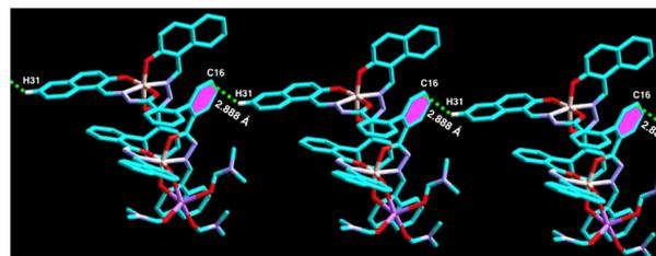
Fig. 3 Perspective views of C–H... $\pi$ (C) interactions of complex 1.
