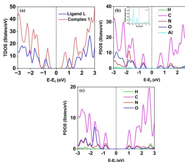
Fig. 10 (a) Total density of states (TDOS) spectrum of ligand **L** and complex **1**, the partial density of states (PDOS) spectrum of (b) complex **1**, and (c) ligand **L**. The black dotted line indicates the Fermi level ( $E_f$ ).
