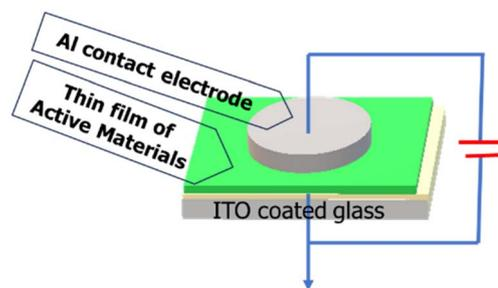
Scheme 1 Schematic of metal–semiconductor junction for electrical measurements.
