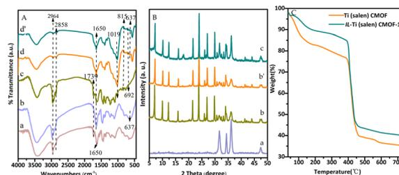
Fig. 1 FT-IR spectra of the Ti(salen)-derived dicarboxylic bridging linker (A-a), Ti(salen) CMOF (A-b), IL-Ti(salen)-derived dicarboxylic bridging linker (L<sub>1</sub>) (A-c), the fresh IL-Ti(salen) CMOF-1 (A-d) and the reused IL-Ti(salen) CMOF-1 (A-d'); PXRD patterns of Ti(salen) CMOF (B-a), IL-Ti(salen) CMOF-1 (B-b), the reused IL-Ti(salen) CMOF-1 (B-b') and IL-Ti(salen) CMOF-2 (B-c); TGA (C) analysis of Ti(salen) CMOF and IL-Ti(salen) CMOF-1.
