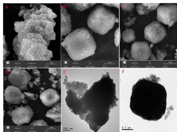
Fig. 2 SEM images of **Ti(salen) CMOF** (A), fresh **IL-Ti(salen) CMOF-1** (B), reused **IL-Ti(salen) CMOF-1** (C), **IL-Ti(salen) CMOF-2** (D); TEM images of **Ti(salen) CMOF** (E) and **IL-Ti(salen) CMOF-1** (F).
