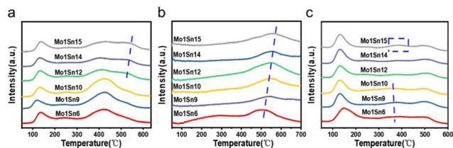
Fig. 5 (a) O<sub>2</sub>-TPD spectra of catalysts with different Mo–Sn ratios, (b) CO<sub>2</sub>-TPD spectra of catalysts with different Mo–Sn ratios, and (c) NH<sub>3</sub>-TPD spectra of catalysts with different Mo–Sn ratios.
