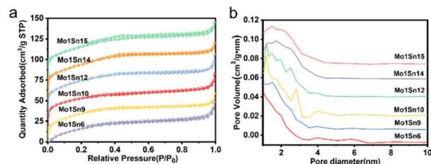
Fig. 1 (a) N<sub>2</sub> adsorption-desorption isotherms of catalysts with different Mo–Sn ratios, (b) pore size distribution of catalysts with different Mo–Sn ratios.
