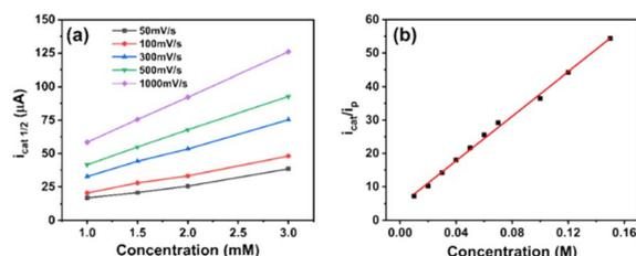
Fig. 6 Plot of  $i_{\text{cat}1/2}$  (half-way catalytic current) in the function of the concentration of NiL complex at different potential scan rates in the presence of  $70 \text{ mM}$  acetic acid as the proton source (a). A plot of  $i_{\text{cat}}/i_p$  as a function of acetic acid concentration while using  $1 \text{ mM}$  NiL, the potential scan rate of  $50 \text{ mV s}^{-1}$  (b).
