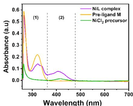
Fig. 1 UV-vis spectra recorded for NiL complex, Ni-precursor and the free ligand dissolved in DMF solution.
