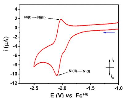
Fig. 3 Cyclic voltammograms recorded on a stationary glassy carbon electrode for the 1 mM NiL in DMF solution. The potential scan rate was 50 mV s<sup>-1</sup>.
