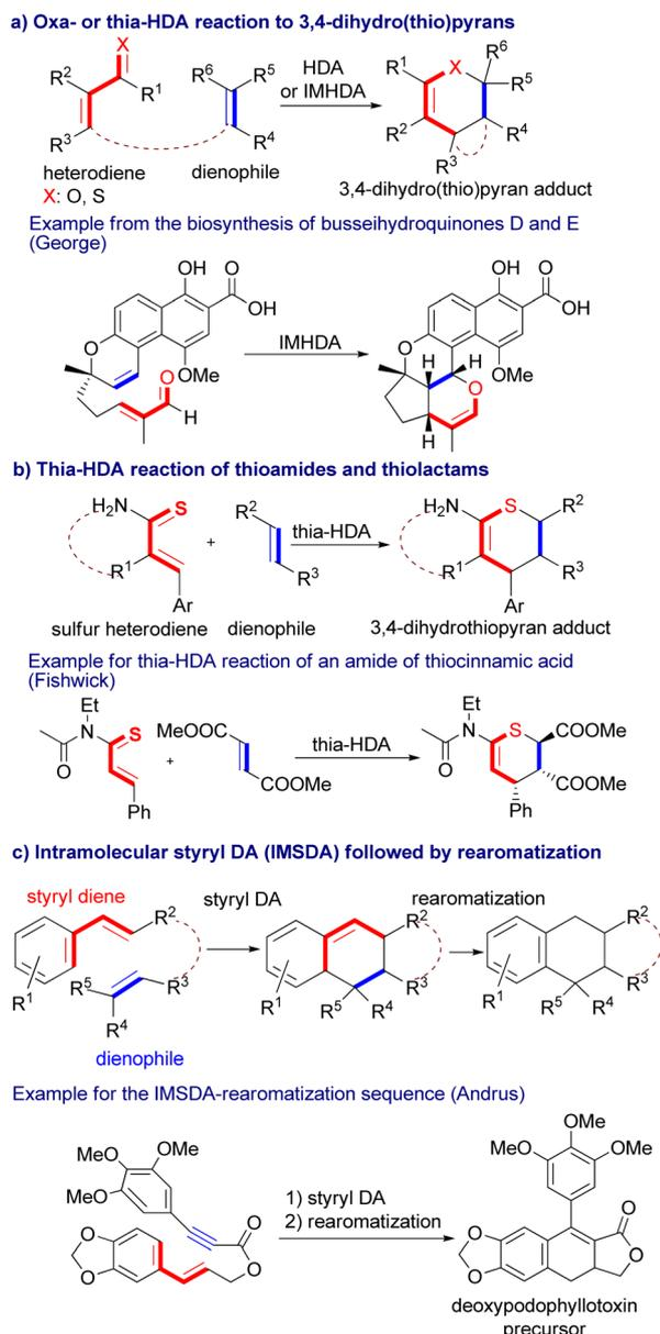
**Scheme 1** (a) General scheme for oxa- and thia-HDA and an example for an IMHDA cyclization. (b) General scheme for the thia-HDA reaction of thioamides and thiolactams with an example for amides of thiocinnamic acid. (c) General scheme and a specific example for IMSDA reactions.
