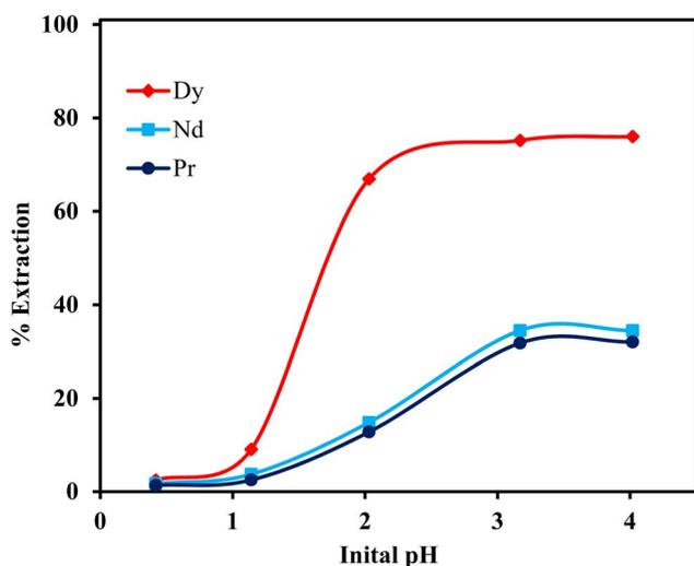
Fig. 8 Effect of initial pH on the extraction of Dy(III), Nd(III), and Pr(III). Aqueous phase:  $[Dy^{3+}] = 0.12 \text{ g L}^{-1}$ ,  $[Nd^{3+}] = 1.63 \text{ g L}^{-1}$  and  $[Pr^{3+}] = 0.44 \text{ g L}^{-1}$ . Organic phase:  $0.01 \text{ mol L}^{-1}$  [P66614][Cy272] ionic liquid, O/A = 1 : 1.
