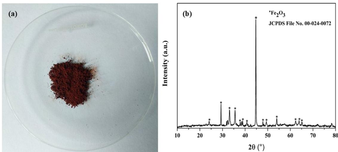
Fig. 6 (a) Image of iron precipitate as hematite and (b) XRD graph of Fe<sub>2</sub>O<sub>3</sub>.
