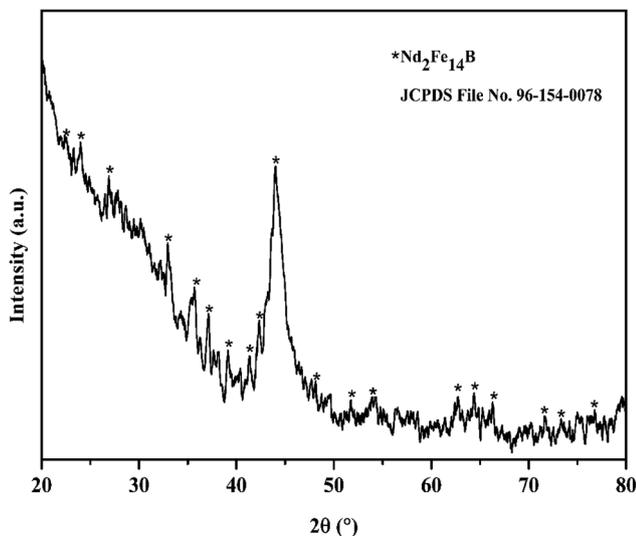
**Fig. 2** XRD graph of waste HDDs magnet sample.
