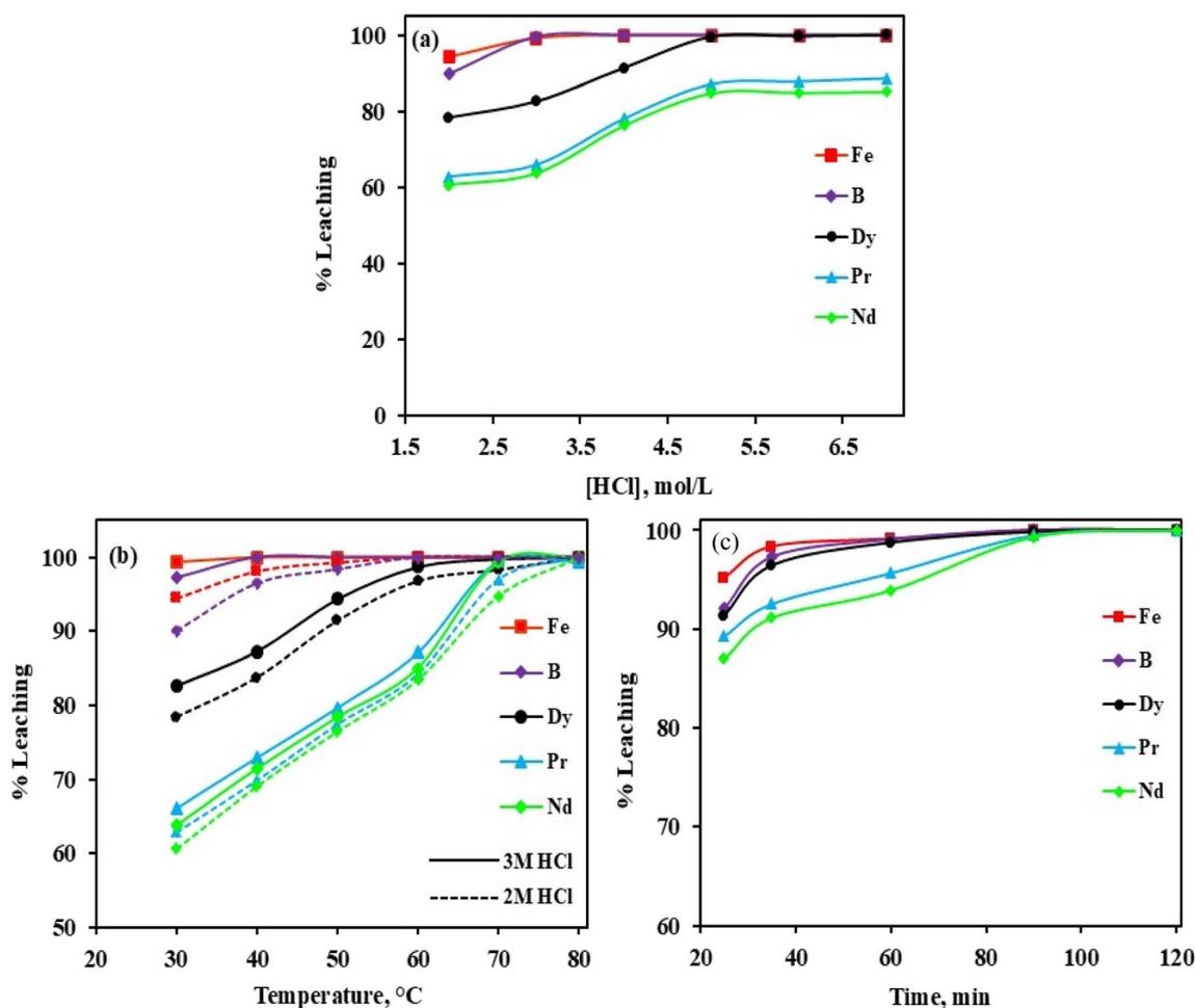
Fig. 5 Effect of various parameters on leaching efficiency of REEs, B and Fe, (a) HCl concentration (temperature = 30 °C, PD = 10 g L<sup>-1</sup>, leaching time = 90 min, rpm = 400), (b) temperature ([HCl] = 2 mol L<sup>-1</sup> and 3 mol L<sup>-1</sup>, PD = 10 g L<sup>-1</sup>, leaching time = 90 min, rpm = 400) and (c) leaching time ([HCl] = 2 mol L<sup>-1</sup>, PD = 10 g L<sup>-1</sup>, temperature = 80 °C, rpm = 400).
