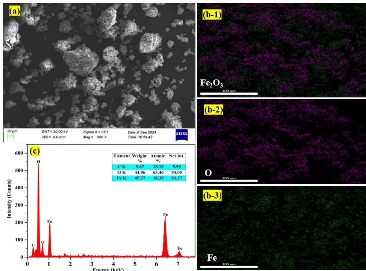
Fig. 7 (a) SEM image, (b) elemental mapping and (c) EDS plot of Fe<sub>2</sub>O<sub>3</sub>.
