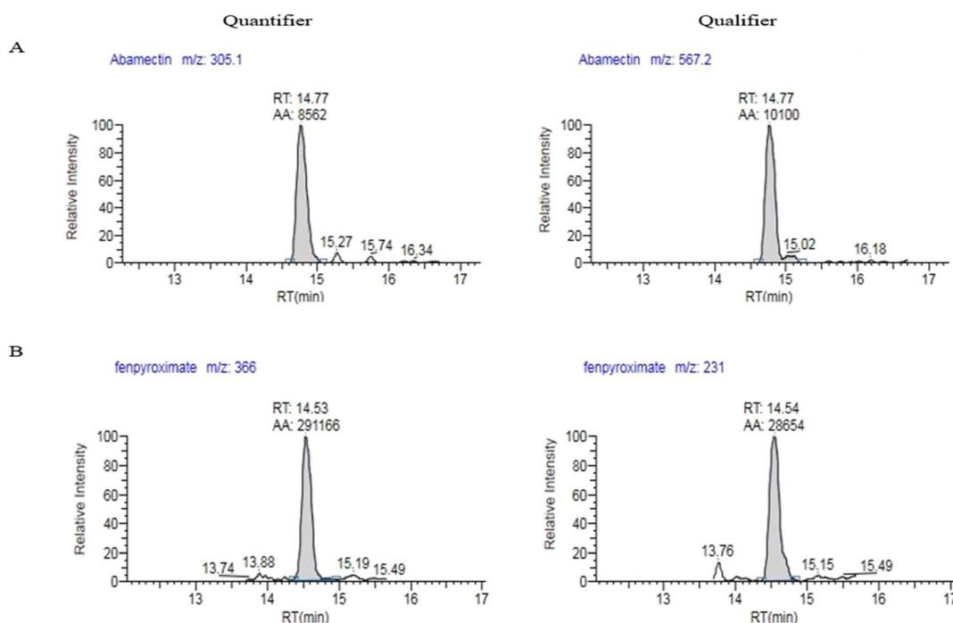
Fig. 3 Product ion chromatograms ( $m/z$ ) for abamectin (A) and fenpyroximate (B) in the spiked okra matrix at 0.005 mg kg<sup>-1</sup>.
