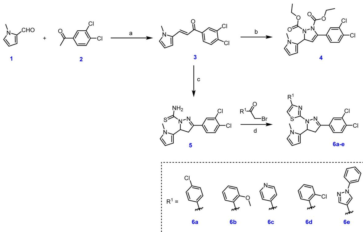
**Scheme 1** Synthesis of target compounds **4**, and **6a–e**. Reagents and conditions: (a) NaOH (10% aq.), EtOH, 0 °C–rt, 4 h; (b) diethyl azodicarboxylate,  $\text{Ph}_3\text{P}$ , toluene, rt, 7h, 60%; (c) thiosemicarbazide, NaOH, EtOH, 100 °C, 8 h, 87%; (d) phenacyl bromide derivative, EtOH, 100 °C, 3h, 49–88%.
