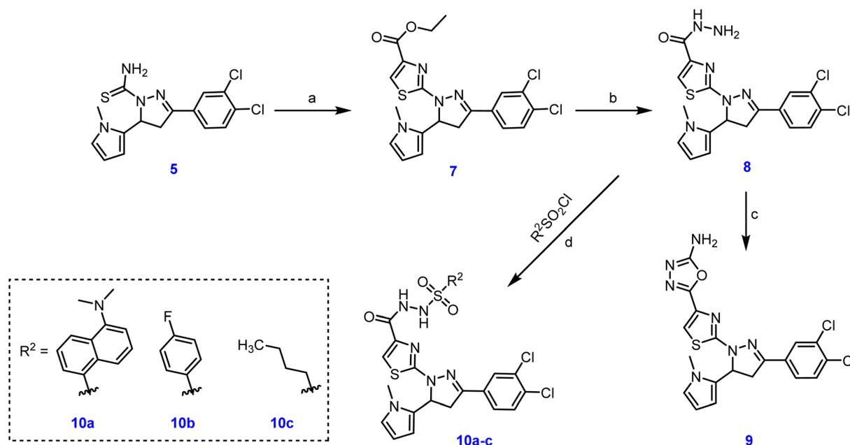
Scheme 2 Synthesis of target compounds **9**, and **10a–c**. Reagents and conditions: (a)  $\alpha$ -bromopyruvate, EtOH, 60 °C, 4 h, 88%; (b) hydrazine hydrate, EtOH, 100 °C, 5h, 89%; (c) (1) cyanogen bromide, MeOH, 1,4-dioxane, rt, 1 h (2)  $\text{NaHCO}_3$ , rt, 18 h, 73%; (d) aryl sulfonyl chloride, DMF, 0 °C–rt, 4–10 h, 65–84%.
