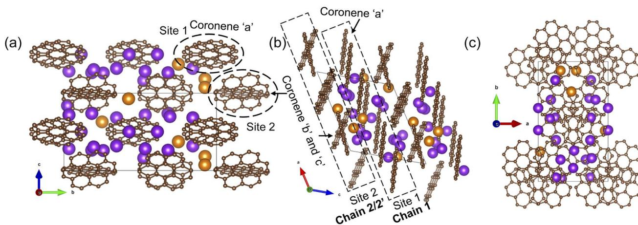
Fig. 5 (a)–(c) A locally represented model of the structure of  $K_{3.03(3)}$ coronene, derived from the disordered refined  $K_{3.03(3)}$ coronene model. The rounding of K occupancies when assembling the local representation gives the composition  $K_{3.125}$ coronene. Brown and pink spheres represent carbon and hydrogen, respectively. Purple and orange spheres represent  $K^+$  ions present within a chain and between the chains, respectively (see Fig. 6).
