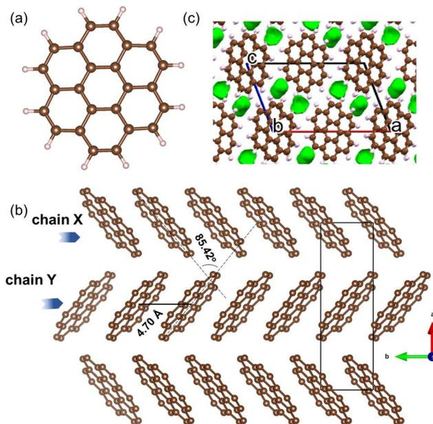
Fig. 2 (a) Molecular structure of coronene ( $C_{24}H_{12}$ ). Brown and light pink spheres represent carbon and hydrogen atoms, respectively. (b) Herringbone packing of coronene viewed along the crystallographic  $c$ -direction with hydrogen atoms omitted. (c) Void space in crystalline coronene computed and plotted using Mercury<sup>20</sup> with a probe radius of 0.65 Å, showing voids lie between the chains.
