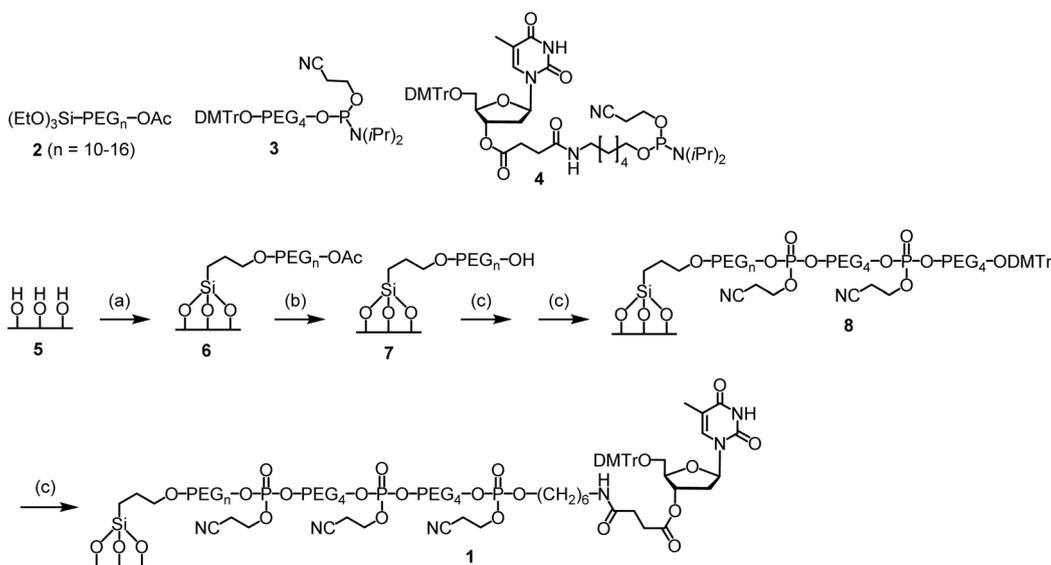
**Scheme 2** Functionalization of glass wool and glass beads. Conditions: (a) **2** (1% PhMe), rt, 20 min; then, supernatant removed, glass wool 100 °C, 4 h. (b) NH<sub>4</sub>OH (30%), 55 °C, 2 h. (c) On a DNA synthesizer, standard coupling, oxidation and deblocking conditions with modifications; see the ESI† for details.
