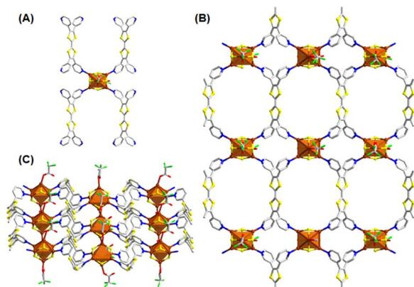
Fig. 5 Structural architecture of  $\text{Cu}_6$ -dpp (A)  $\text{Cu}_6$  cluster node geometry and the attachment of four thiolate groups,  $\text{CF}_3\text{COO}^-$  units and the attachment of linker molecules, (B) 2D architecture of the  $\text{Cu}_6$ -dpp CAM (C) ladder-like architecture. Hydrogen atoms and the associated solvent molecules are removed for the clarity. Color legend: Cu, brown; S, yellow; O, red; F, green; N, blue; C, grey stick.
