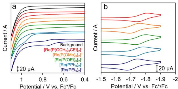
Fig. 2 Cyclic voltammograms of  $[\text{Re}(\text{PR}_3)_2]^+$  (0.5 mM) acquired at  $200 \text{ mV s}^{-1}$  in Ar-saturated DMA containing  $\text{Et}_4\text{NBF}_4$  (0.1 M) using a glassy-carbon working electrode (diameter: 3 mm) and a Pt-wire counter electrode: (a) oxidation and (b) reduction sides.
