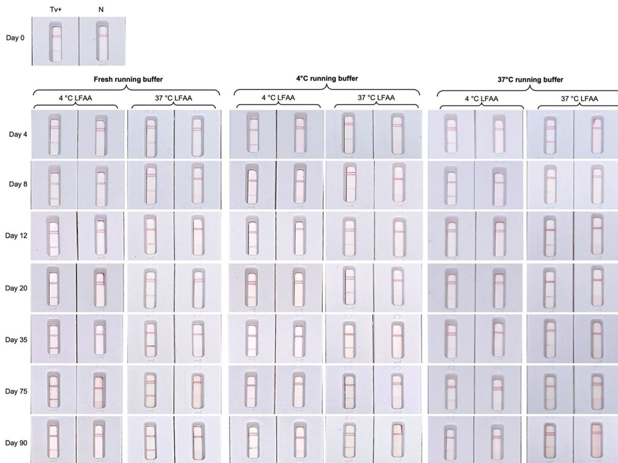
Fig. 6 Stability of the ALFA and the running buffer stored at 4 °C and 37 °C. Representative of duplicate tests. Legend: Tv+ =  $4.0 \times 10^6$  lysed *T. vaginalis* cells per mL, N = negative/sample buffer only.
