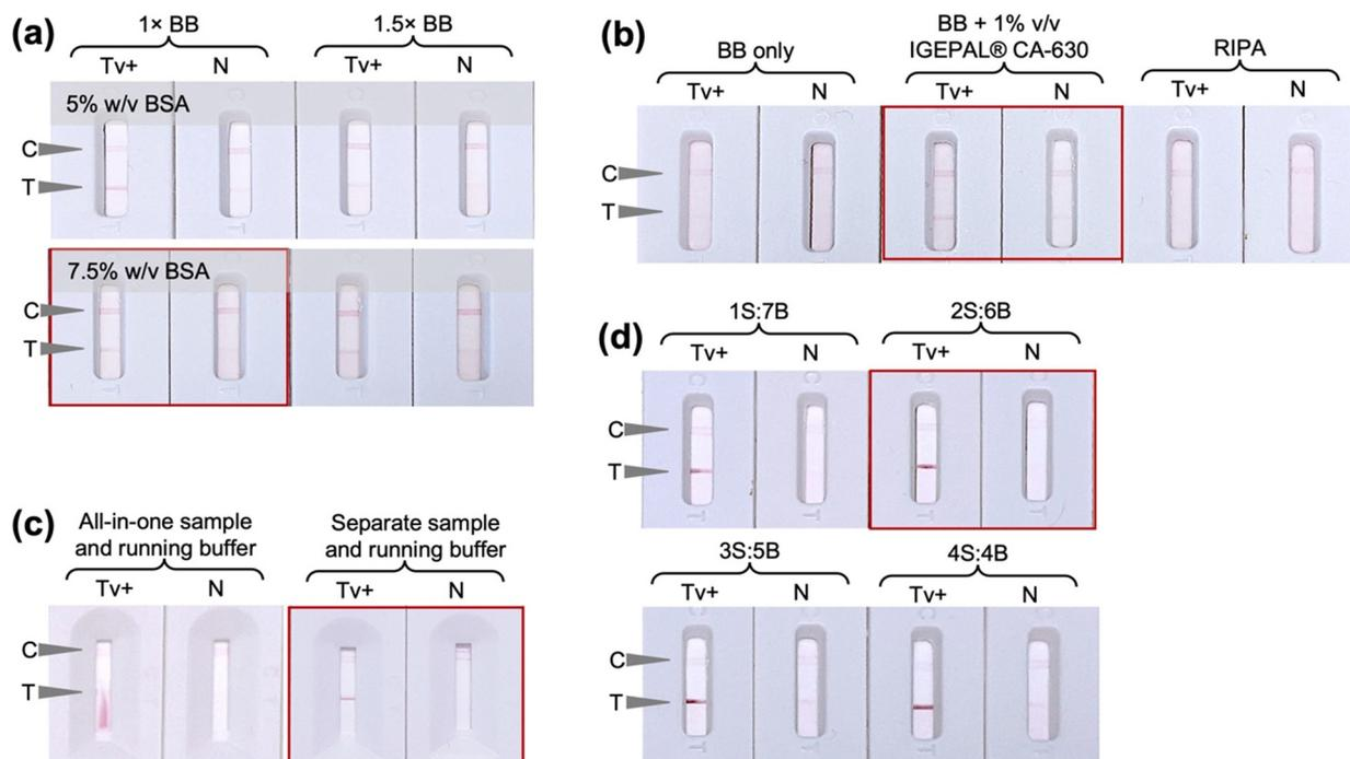
**Fig. 5** Optimization of ALFA buffers. (a) Running buffer; (b) sample buffer; (c) use of combined or separate sample and running buffers; (d) dilution of lysed sample with running buffer at 1:7 – 4:4 ratios of sample:running buffer. Legend: C = control zone, T = test zone, Tv+ =  $4.0 \times 10^6$  cells per mL of *T. vaginalis* in lysis solution, N = negative/sample buffer only, BB = binding buffer, S = sample in lysis buffer, B = running buffer.
