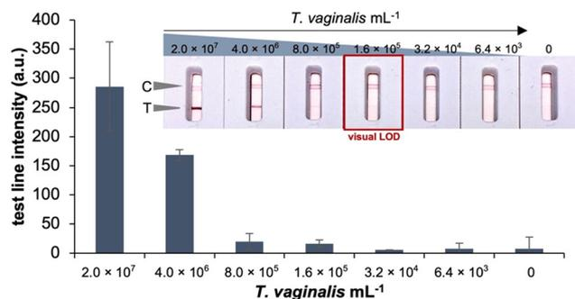
**Fig. 7** Calibration curve of ALFA using serially diluted *T. vaginalis* cells in sample buffer. The error bars correspond to the variation from duplicate sample analysis. Test line intensities measured using the Cube LFA reader (Biosynex Technologies, Germany). Legend: C = control zone, T = test zone, N = negative/sample buffer only, a.u. = arbitrary unit.
