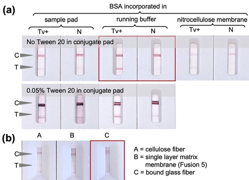
**Fig. 3** Optimization of ALFA components. (a) Use of Tween 20 and BSA in different components of the ALFA was tested in the presence (Tv+) and absence (N) of *T. vaginalis* cells; (b) choice of sample pad material using only blank sample buffer mixed with running buffer. Legend: C = control zone, T = test zone, Tv+ =  $4.0 \times 10^6$  cells per mL of *T. vaginalis* in lysis solution, N = negative/sample buffer only.
