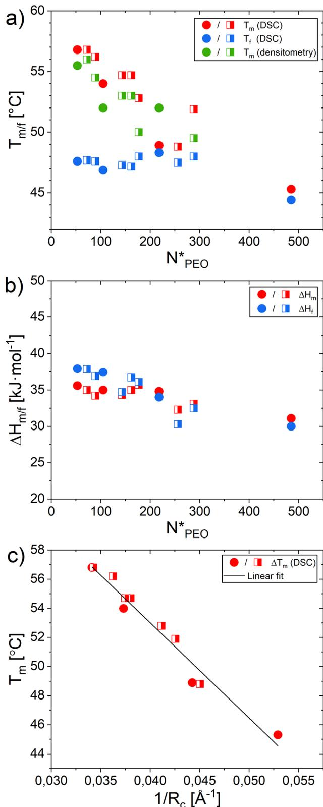
Fig. 6 (a) Melting/freezing points  $T_m/T_f$  determined from DSC as well as  $T_m$  from densitometry plotted against the mean PEO block length  $N_{PEO}^*$ . (b) melting/freezing enthalpies  $\Delta H_m/\Delta H_f$  determined from DSC plotted against the mean PEO block length  $N_{PEO}^*$ . (c) Melting temperature of the C<sub>28</sub> alkyl core blocks plotted against the inverse core radius  $1/R_c$ . The solid line is a linear fit with a coefficient of determination  $R^2$  of 0.96.
