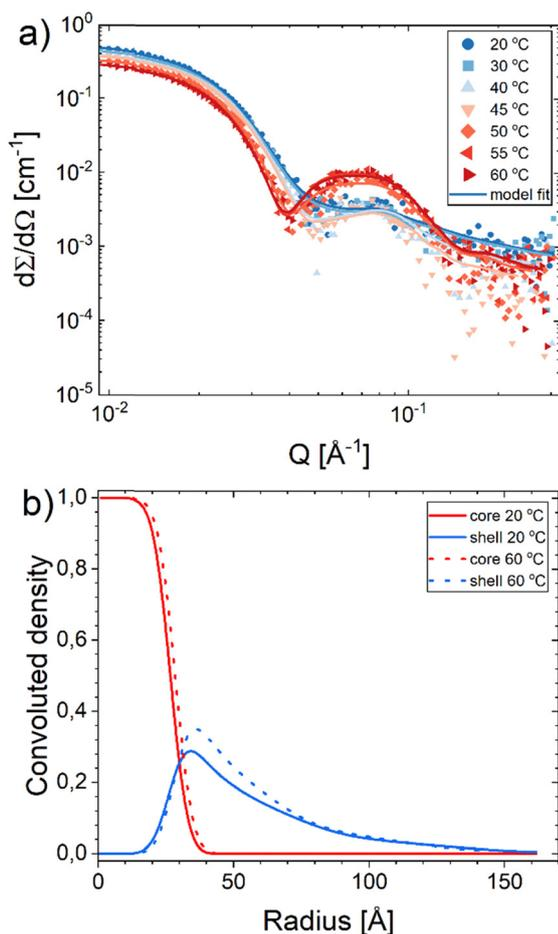
**Fig. 3** (a) SAXS curves of  $C_{28}$ -PEO3/10 1:1 as a function of temperature ranging from 20 °C to 60 °C at 0.5 vol% polymer concentration. Solid lines represent the model fits. Temperature scans of other samples can be found in Fig. S2 and S3 in the ESI.† (b) The density profile of core (red) and shell (blue) as a function of micelle radius of  $C_{28}$ -PEO3/10 1:1 micelles at 20 °C (solid line) and 60 °C (dotted line).
