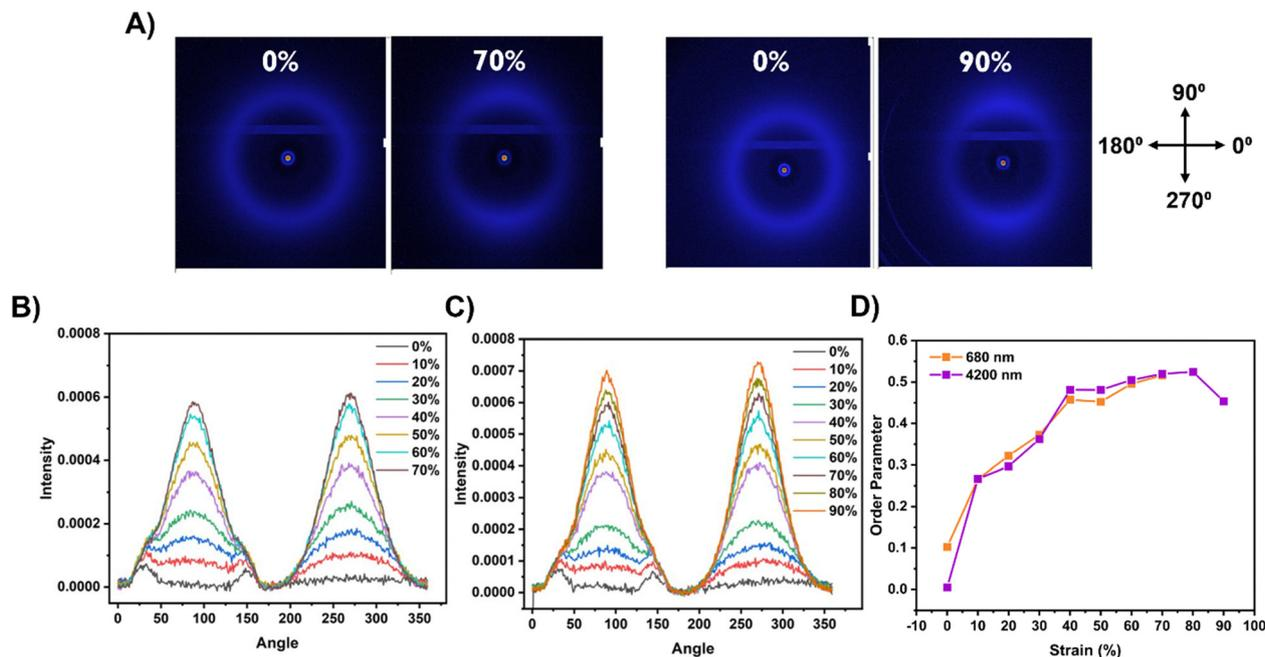
Fig. 6 (A) WAXS scattering patterns of 50  $\mu\text{m}$  thick visible (left pair) and MWIR (right pair) CLCEs before and after strain. Scattering intensity vs. angle for (B) visible reflective CLCE and (C) a MWIR reflective CLCE. (D) Calculated order parameter for visible and MWIR reflective CLCEs under strain.
