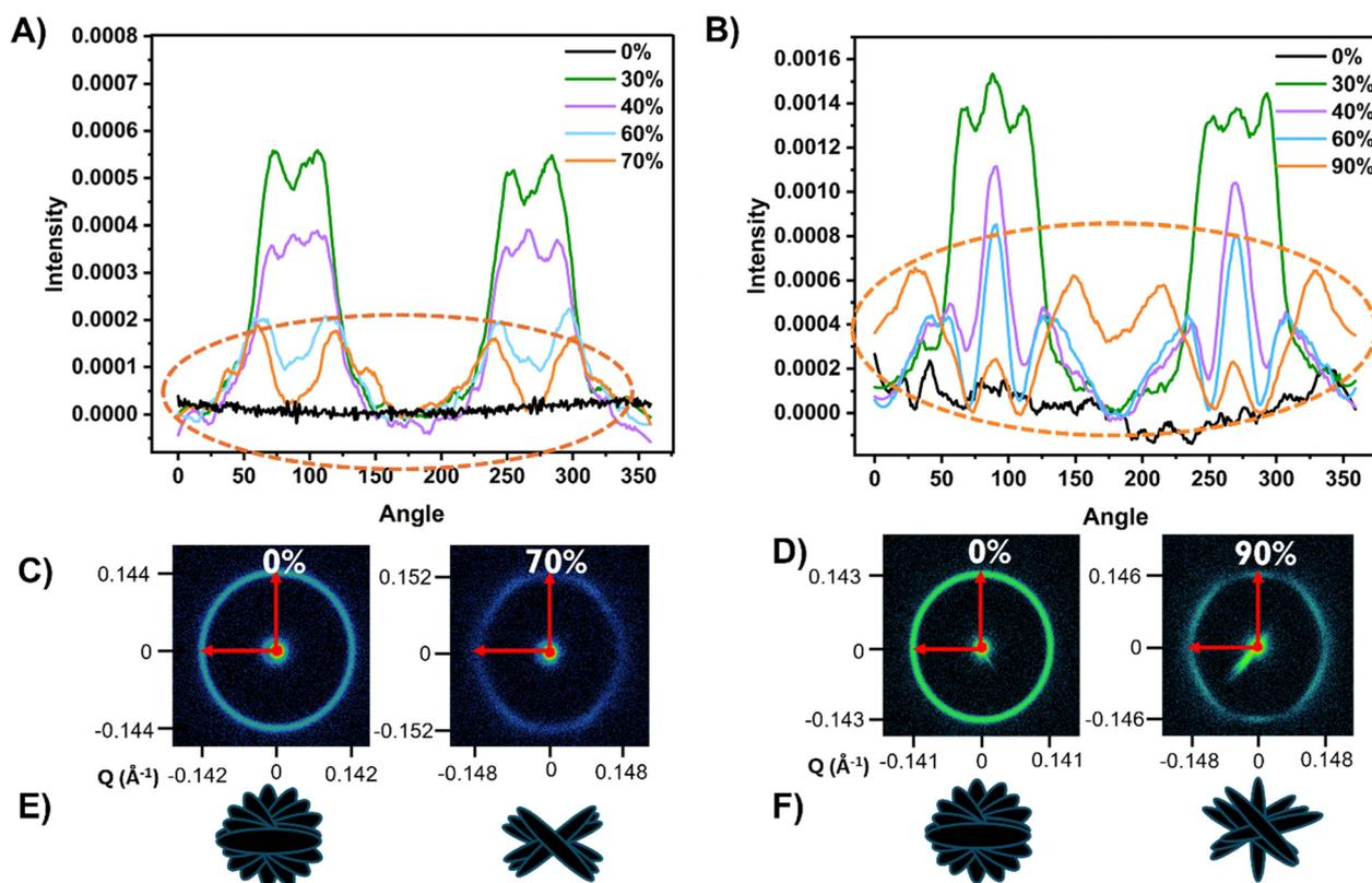
Fig. 7 (A) SAXS intensity vs. angle of 50  $\mu\text{m}$  thick (A) visible and (B) MWIR reflective CLCEs under strain. SAXS scattering patterns of a (C) visible CLCE at 0% and 70% strains and (D) of a MWIR CLCE at 0% and 90% strains. Depictions of the LC director reorientation and distortion is represented for (E) visible and (F) MWIR reflective CLCEs before and after strain.
