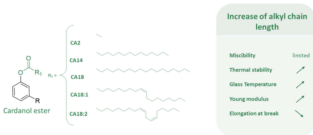
Fig. 5 Study of cardanol esters: influence of the alkyl chain length on plasticized PVC material properties.
