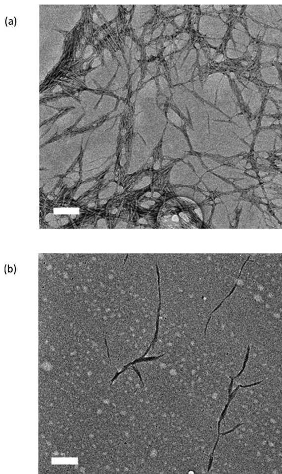
Fig. 3 TEM images of (a) wet NCC (W-NCC) and (b) spray-dried NCC (SD-NCC) at 100 00 $\times$  magnification.
