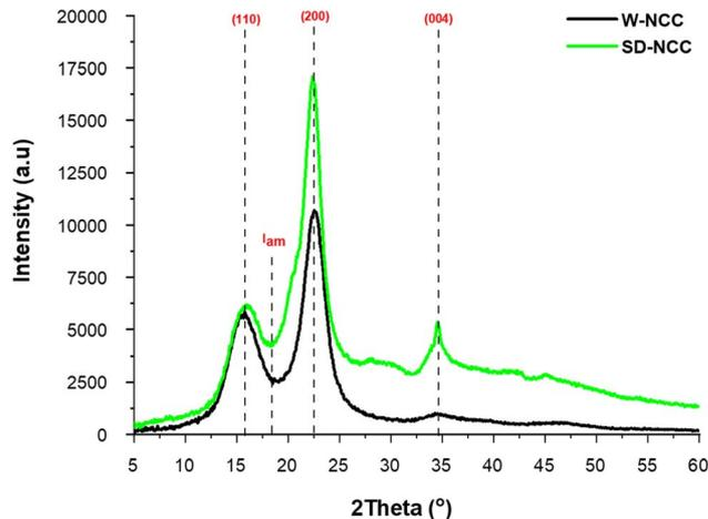
Fig. 4 XRD spectra of W-NCC and SD-NCC.
