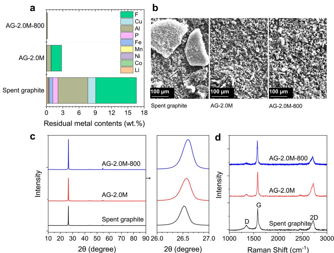
Fig. 5 Characterisation of recovered graphite. (a) Residual metal contents after optimized recycling processes. (b) SEM images. (c) XRD spectra. (d) Raman spectra. AG-2.0M: graphite recovered via 2 M  $\text{H}_2\text{SO}_4$  leaching. AG-2.0M-800: graphite recovered via 2 M  $\text{H}_2\text{SO}_4$  leaching followed by 800 °C pyrolysis.
