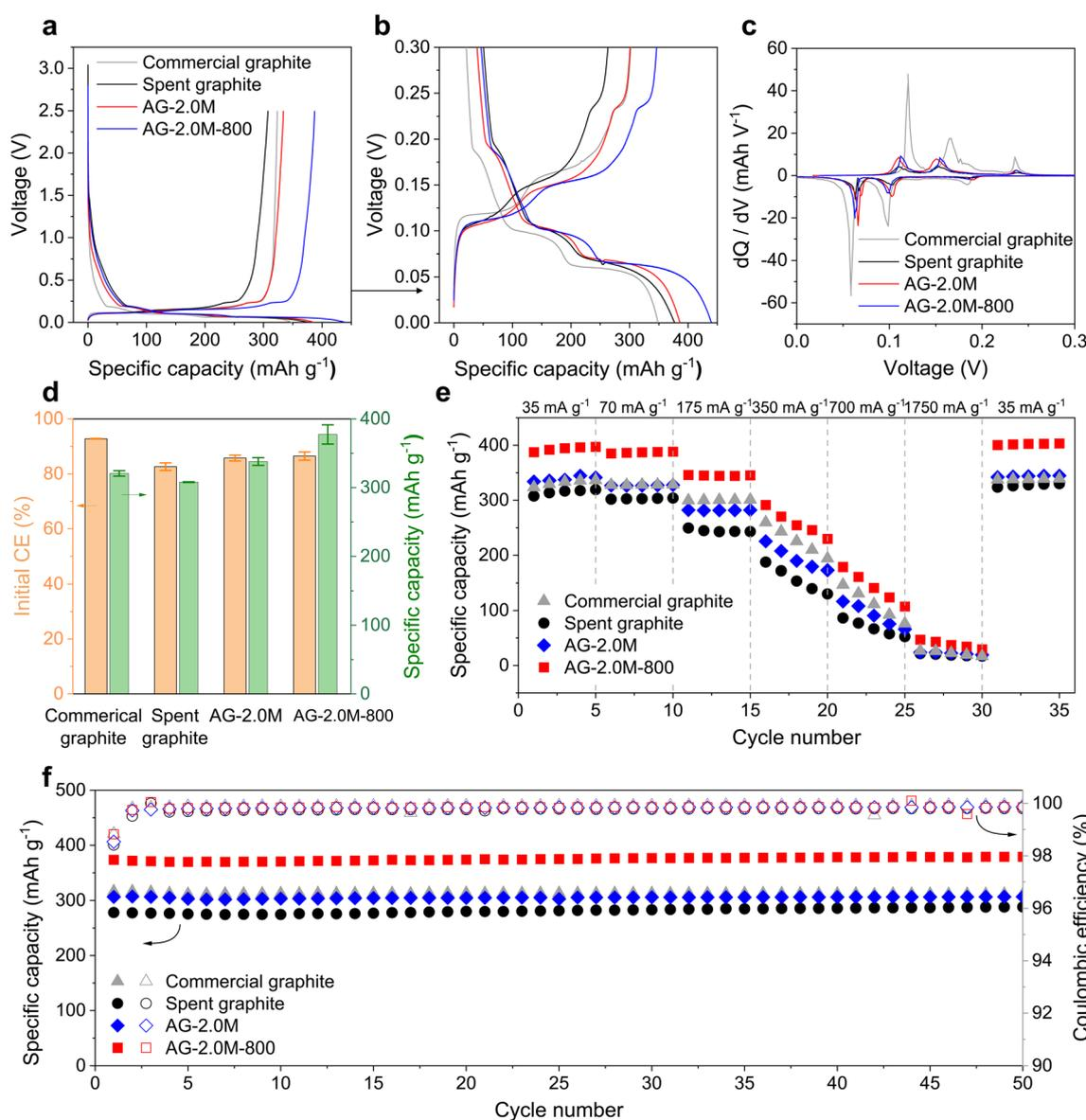
Fig. 7 Electrochemical performance of recovered graphite. (a and b) Charge–discharge profiles of the first cycle at 0.1C. (c)  $dQ/dV$  profiles. (d) Summary of the initial CEs and charge capacities. Error bars represent standard deviation based on three independent cells. (e) Rate performance. (f) Cycling performance in a half-cell configuration at 0.5C (175  $\text{mA g}^{-1}$ ).
