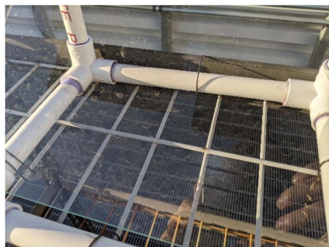
Fig. 6 Image of control panel dust buildup after 10 days of outdoor exposure.
