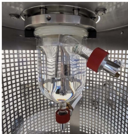
Fig. 1 Glass reactor (Büchi) with a built-in pitched blade stirrer, a thermocouple, immersion tubes and a baffle.
