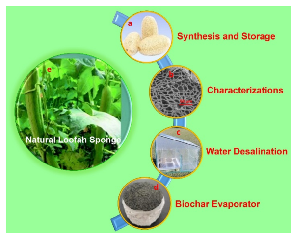
Fig. 1 Contents of the present review. (a) Digital photograph of dried loofah sponge. Reproduced with permission from ref. 58. Copyright (2023) Elsevier Inc. (b) Cross-sectional SEM image of inner side of loofah fiber. Reproduced with permission from ref. 58. Copyright (2023) Elsevier Inc. (c) Digital photo of an outdoor water desalination setup. Reproduced with permission from ref. 58. Copyright (2023) Elsevier Inc. (d) Loofah sponge biochar evaporator. Reproduced with permission from ref. 42. Copyright (2022) Elsevier Inc. (e) Digital image of loofah plant. Reproduced with permission from ref. 61. Copyright (2020) Royal Society of Chemistry.
