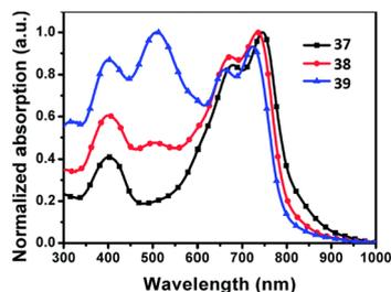
Fig. 7 Absorption spectra of terpolymers 37–39 as thin films. Copyright 2014 (RSC).<sup>75</sup>
