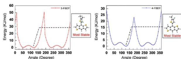
Fig. 10 Torsional energy profiles of thienyl-BDT with F on different positions of the thienyl side chain. Copyright 2023 (RSC).<sup>86</sup>
