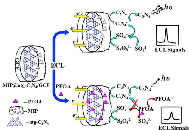
Fig. 13 Illustrative electrochemiluminescence detection technique for PFOA with MIP-functionalized utg- $C_3N_4$  in  $S_2O_8^{2-}$  system. Reproduced from ref. 105 Copyright 2015, Elsevier.
