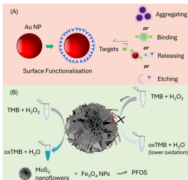
Fig. 5 (A) Illustration of the possible interactions between Au NPs and the target analyte. Reproduced from ref. 64 Copyright 2017, Elsevier. (B) MoS<sub>2</sub>/Fe<sub>3</sub>O<sub>4</sub> nano-flowers for the colorimetric determination of PFAS producing a blue hue when 3,3,5,5-tetramethylbenzidine (TMB) is oxidized in H<sub>2</sub>O<sub>2</sub>. Reproduced from ref. 65 Copyright 2019, Elsevier.
