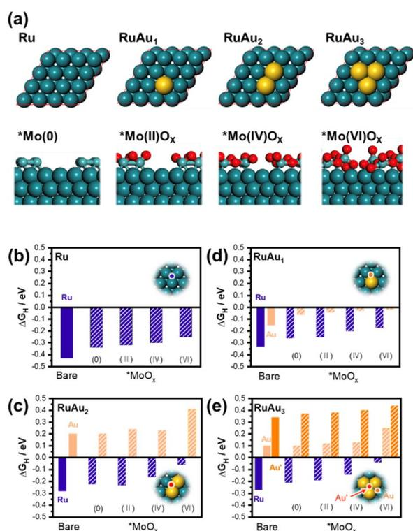
Fig. 5 (a) Atomic structures of RuAu surfaces with varying Au content and adsorbed  $\text{MoO}_x$  clusters with different oxidation states. H-binding free energies ( $\Delta G_{\text{H}}$ ) for various active sites on (b) Ru, (c)  $\text{RuAu}_2$ , (d)  $\text{RuAu}_1$ , and (e)  $\text{RuAu}_3$  surfaces with and without  $\text{MoO}_x$  clusters. Blue bars represent Ru sites, orange bars represent Au sites, and hatched bars indicate sites affected by  $\text{MoO}_x$ .
