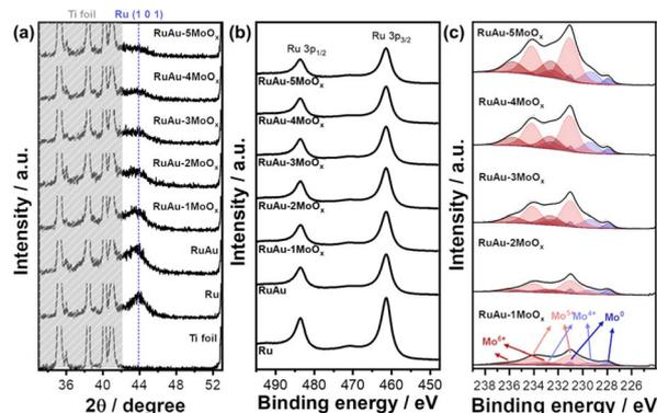
Fig. 3 (a) X-ray diffraction patterns of Ru, RuAu, and RuAu-1–5MoO<sub>x</sub> deposits on Ti foil. (b) Ru 3p XPS spectra and (c) Mo 3d XPS spectra of RuAu-1–5MoO<sub>x</sub> deposits on Ti foil.
