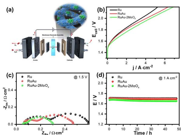
Fig. 6 Electrochemical measurements for Ru, RuAu, and RuAu-2MoO<sub>x</sub> as the electrocatalyst for the HER in PEMWE. (a) Schematic diagram of the PEMWE unit cell with the RuAu-MoO<sub>x</sub> electrocatalyst. (b) *j*-*V* curves of the PEMWE cell. (c) Nyquist plots with an amplitude of 18 mV and an applied voltage of 1.5 V. (d) Chronopotentiometry response at a current density of 1 A cm<sup>−2</sup> during 48 hours of operation.
