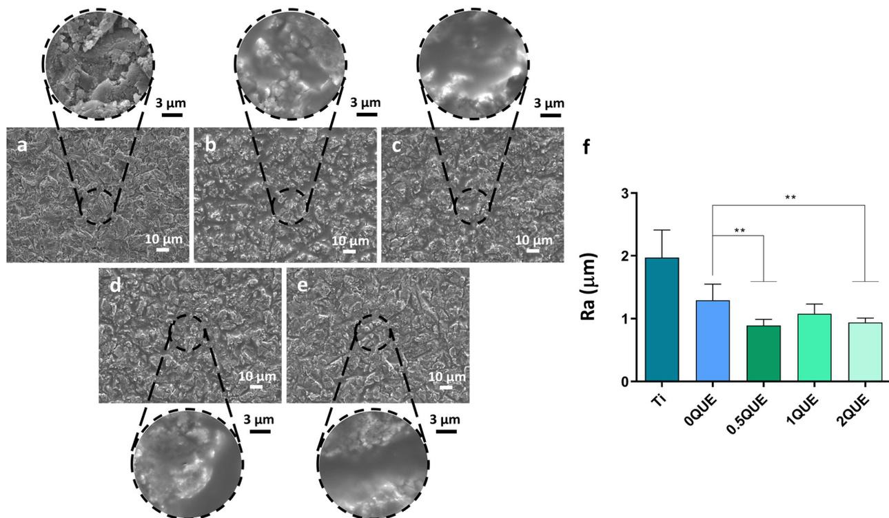
Fig. 1 SEM micrographs of (a) Ti, (b) 0QUE, (c) 0.5QUE, (d) 1QUE and (e) 2QUE with their respective amplifications. Roughness is shown as the arithmetic average roughness parameter ( $R_a$ ) (f). The asterisks ( $p \leq 0.01$  (\*\*)) indicate statistically significant differences for the QUE-doped coatings in comparison with 0QUE. Results are shown as mean  $\pm$  SD.
