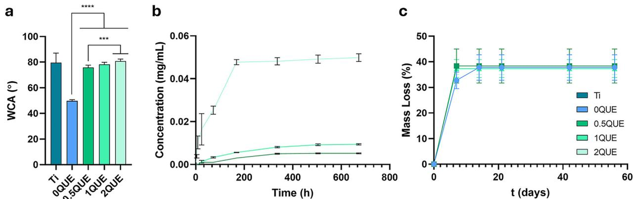
Fig. 3 Contact angle measurements (WCA; (a)), release kinetics of QUE ( $\text{mg mL}^{-1}$ ) (b) and hydrolytic degradation results (c). The asterisks ( $p \leq 0.001$  (\*\*\*) and  $p \leq 0.0001$  (\*\*\*)) indicate statistically significant differences between the QUE-doped coatings and the 0QUE. Results are shown as mean  $\pm$  SD.
