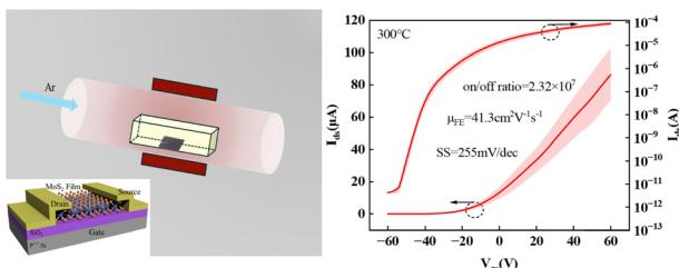
Reducing MoS<sub>2</sub> FET contact resistance by stepped annealing to optimize device performance
