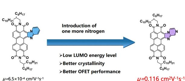
***ortho*- $\pi$ -Extension of perylene diimides via one-pot annulation of imidazo[1,2-a]pyridine or imidazo[1,2-a]pyrazine for n-type organic field-effect transistors**
