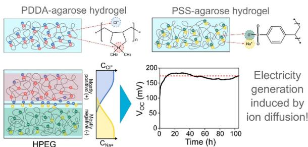
**A hydrogel-ionic polymer blend for humidity-insensitive ion gradient driven electricity generation**
