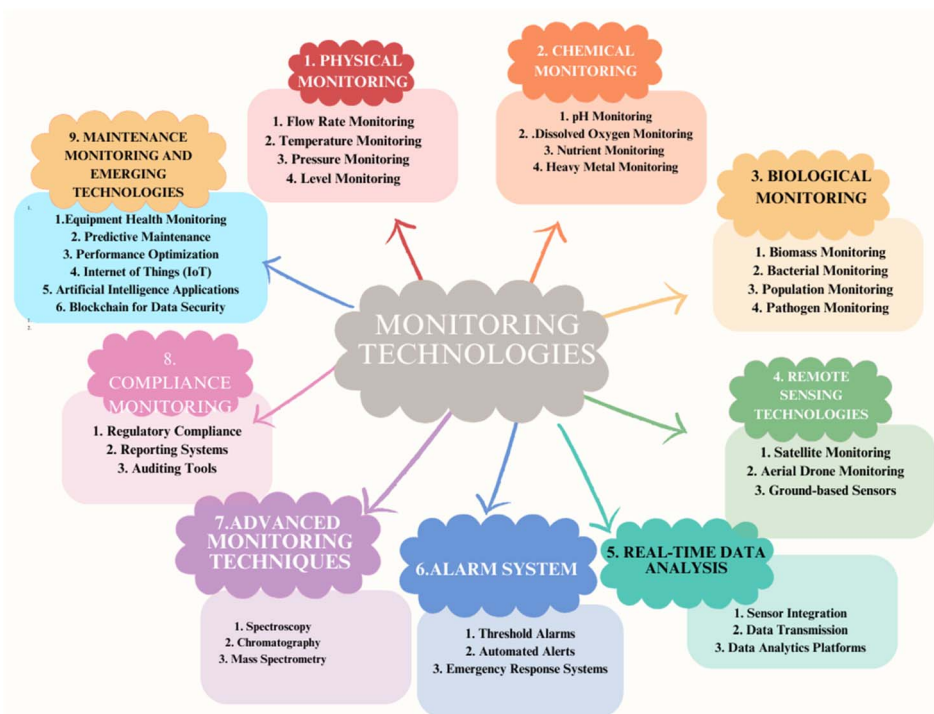
Fig. 26 Monitoring technologies for wastewater treatment plants.
