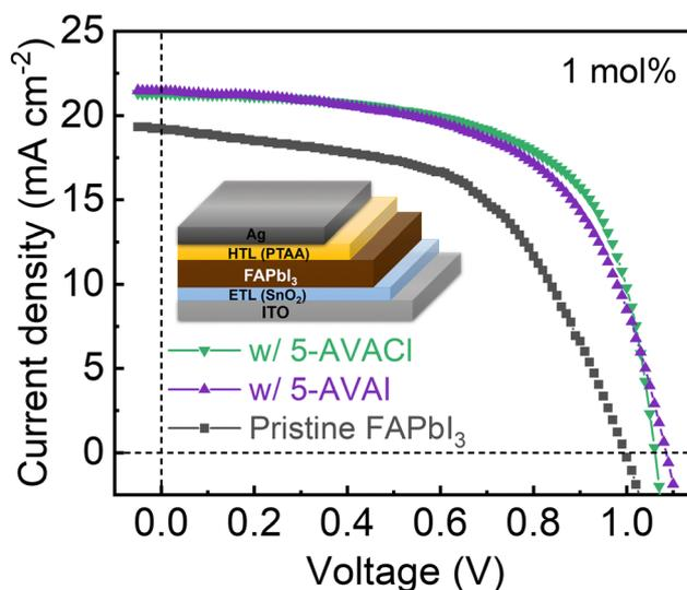
Fig. 6 Forward scan  $J$ - $V$  curves for the champion devices or pristine FAPbI<sub>3</sub>, and FAPbI<sub>3</sub> with 1 mol% 5-AVAI or 5-AVACl added. Inset shows the device structure.
