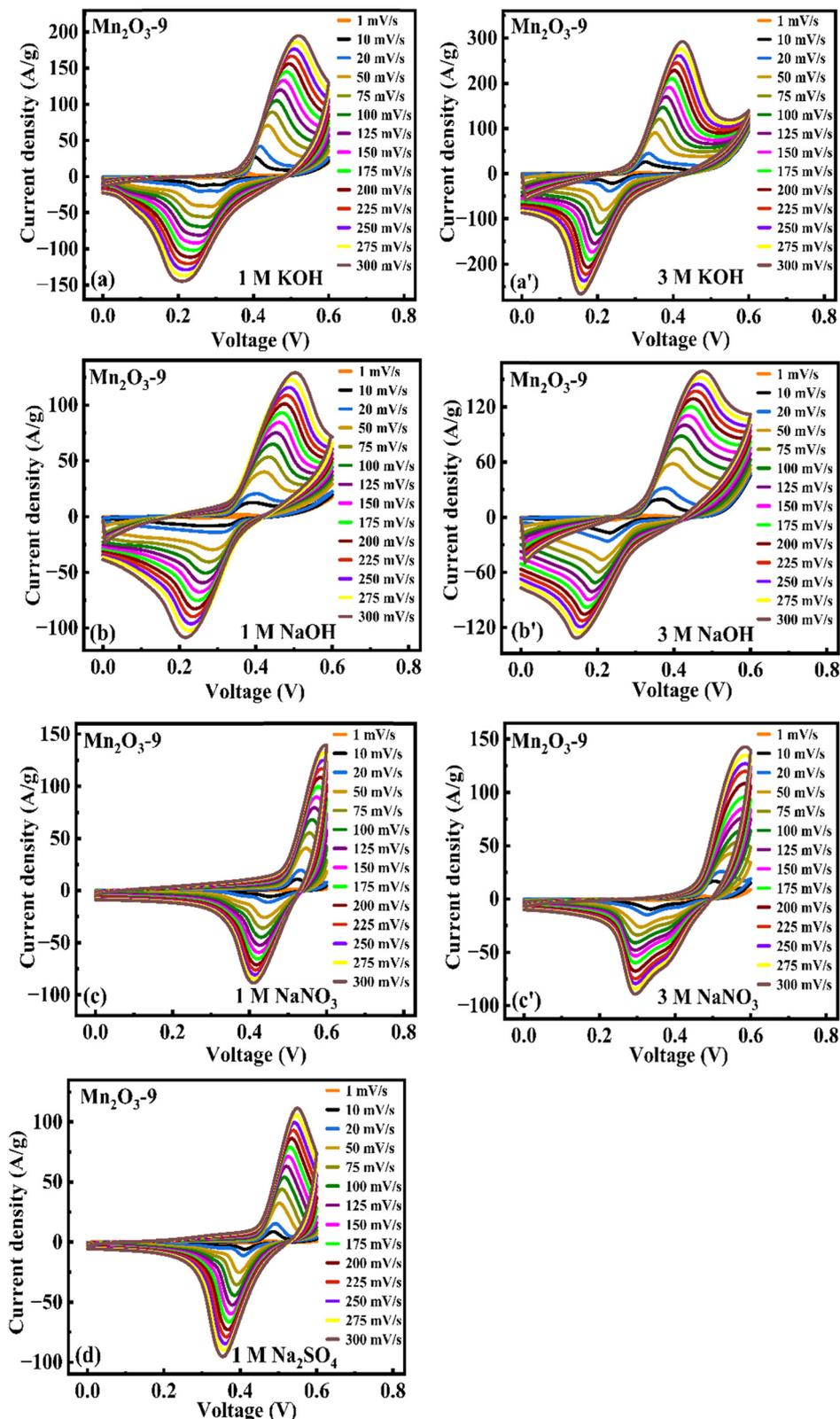
Fig. 9 Cyclic voltammograms of  $\text{Mn}_2\text{O}_3\text{-9}$  at different scan rates in (a)–(d) 1 M and (a')–(c') 3 M concentrations of different electrolytes.
