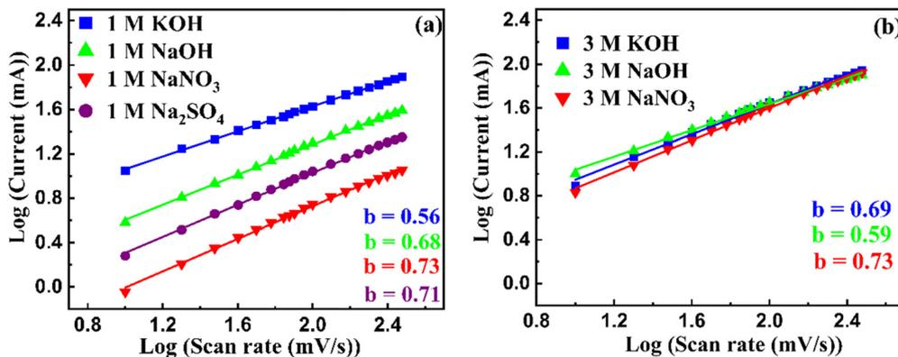
Fig. 10  $b$ -Values plots of Mn<sub>2</sub>O<sub>3</sub>-9 in (a) 1 M and (b) 3 M concentrations of different electrolytes.
