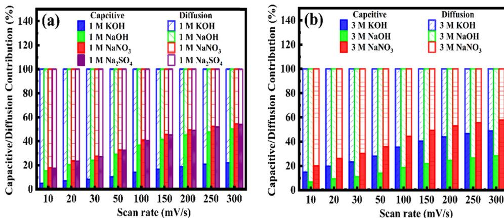
Fig. 12 Percentage capacitive and diffusion contribution to the total charge storage in the Mn<sub>2</sub>O<sub>3</sub>-9 mM urea sample measured in (a) 1 M and (b) 3 M electrolyte concentrations at different scan rates.
