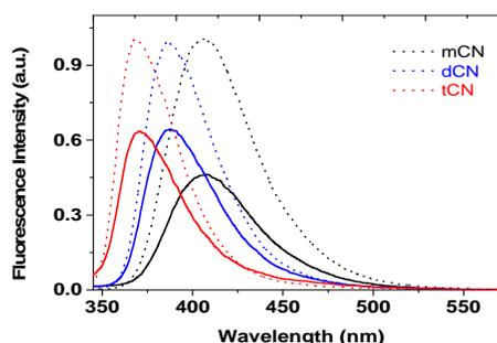
**Fig. 4** Fluorescence spectra of cyanotriphenylamines in toluene (dotted lines) and in toluene with 9.5% polystyrene (solid lines)
