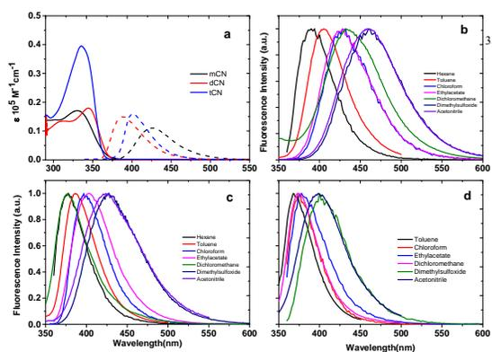
**Fig.2** a) UV-visible absorption (solid line) and fluorescence spectra (dotted line) of cyanotriphenylamine derivatives in toluene. Fluorescence spectra of b) **mCN**, c) **dCN**, and d) **tCN** in different solvents.
