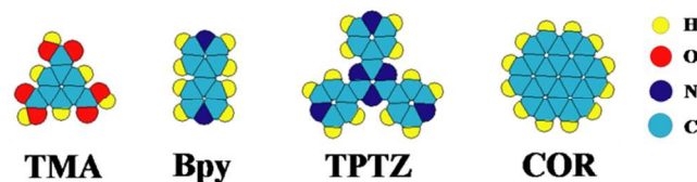
Fig.1 Chemical structures of the adsorbate molecules: 1,3,5-benzenetricarboxylic acid (trimesic acid, TMA, C 9 H 6 O 6 ), 4, 4'-bipyridine (Bpy, C 10 H 10 N 2 ), 1,3,5-tris(4-pyridyl)-2,4,6-triazine (TPTZ, C 18 H 12 N 6 ) and coronene (COR, C 24 H 12 ).
