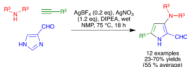
Scheme 75. Silver-promoted, three-component synthesis of pyrroles from secondary amines, alkynes and imidazole-4-carbaldehyde
