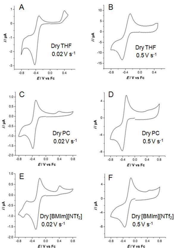
**Fig. 3.** Cyclic voltammetry of  $[\text{Cu}^{\text{II}}(\text{TMPA})(\text{H}_2\text{O})]^{2+}$  ( $\sim 10^{-3}$  mol L $^{-1}$ ) at a glassy carbon disk electrode at 0.02 V s $^{-1}$  (left) and 0.5 V s $^{-1}$  (right) in (A, B) “dry” THF ( $[\text{H}_2\text{O}] = 2.5 \cdot 10^{-3}$  mol L $^{-1}$ ), (C, D) “dry” PC ( $[\text{H}_2\text{O}] = 9.9 \cdot 10^{-3}$  mol L $^{-1}$ ) and (E, F) “dry” [BMIm][NTf $_2$ ] ( $[\text{H}_2\text{O}] = 4 \cdot 10^{-3}$  mol L $^{-1}$ ).
