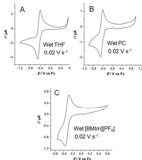
**Fig. 4.** Cyclic voltammetry of  $[\text{Cu}^{\text{II}}(\text{TMPA})(\text{H}_2\text{O})]^{2+}$  ( $\sim 3\text{--}5 \cdot 10^{-3}$  mol L $^{-1}$ ) at a glassy carbon disk electrode at  $\nu = 0.02$  V s $^{-1}$  in (A) “wet” THF ( $[\text{H}_2\text{O}] = 9.5 \cdot 10^{-2}$  mol L $^{-1}$ ), (B) “wet” PC ( $[\text{H}_2\text{O}] = 4.5 \cdot 10^{-1}$  mol L $^{-1}$ ) and (C) “wet” [BMIm][PF $_6$ ] ( $[\text{H}_2\text{O}] = 1.9 \cdot 10^{-1}$  mol L $^{-1}$ ).
