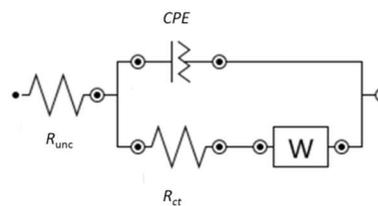
**Scheme 2.** Equivalent circuit used for experimental impedance simulation.  $R_{unc}$ : uncompensated solution resistance;  $R_{ct}$ : charge transfer resistance; CPE: constant-phase element; W: Warburg impedance.
