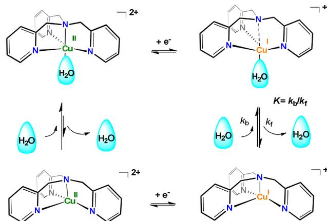
**Scheme 3.** Formal square scheme mechanism for the exchange of water associated with electron transfer for the  $[Cu^{II}(TMPA)(H_2O)]^{2+}$  complex.
