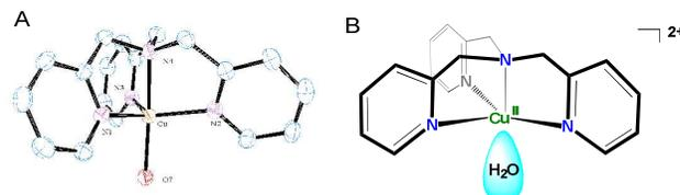
**Fig. 1.** A) ORTEP representation of  $[\text{Cu}^{\text{II}}(\text{TMPA})(\text{H}_2\text{O})](\text{CF}_3\text{SO}_3)_2$  (50 % probability ellipsoids shown). Hydrogen and both triflate anions are omitted for clarity. B) Schematic representation of the  $[\text{Cu}^{\text{II}}(\text{TMPA})(\text{H}_2\text{O})]^{2+}$  complex.
