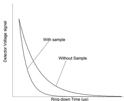
**Figure 1:** Ring-down trace showing exponential decay of the optical signal with and without analyte gas.
