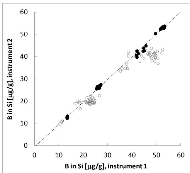
**Figure 5.** Individual ICP-OES B quantification results from table 3 obtained with and without H<sub>2</sub>O<sub>2</sub> addition to sample digests. Data recorded with (●) and without (○) H<sub>2</sub>O<sub>2</sub> added to samples. Dashed line represents a simple, linear regression through data obtained with H<sub>2</sub>O<sub>2</sub> added to samples (regression parameters in table 3).
