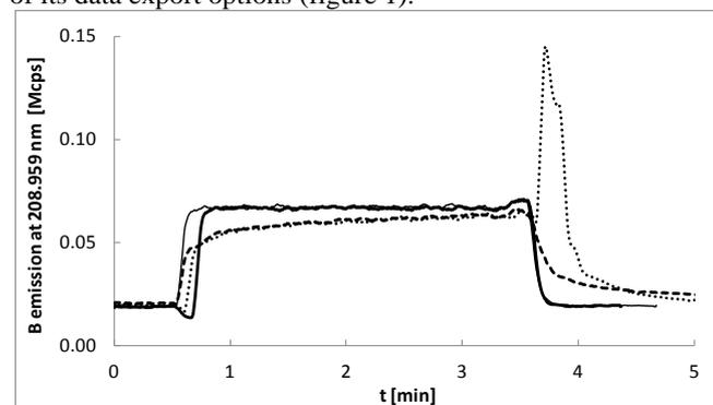
**Figure 1.** Transient B signal profiles of B in a 1 mg/L calibration solution and a digest of MG-Si sample *Elkem 2*. (—) 1 mg/L B calibration solution, rinsed with dilute  $\text{HNO}_3$ . (---) 1 mg/L B calibration solution, rinsed with dilute  $\text{HNO}_3$ /HF blend. (···) *Elkem 2*, rinsed with dilute  $\text{HNO}_3$ . (-·-·) *Elkem 2*, rinsed with dilute  $\text{HNO}_3$ /HF blend.
