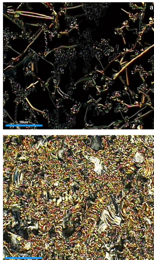
Figure 4 Optical photomicrographs (crossed polarizers along the edges) of a 5\mu\text{m} thick film with planar anchoring of compound IIIc : a) T=162^\circ\text{C} : formation of helical filaments and beaded filaments characteristic of a B7 phase; b) T=145^\circ\text{C} : crystal phasetext of the article should go here with headings as appropriate
