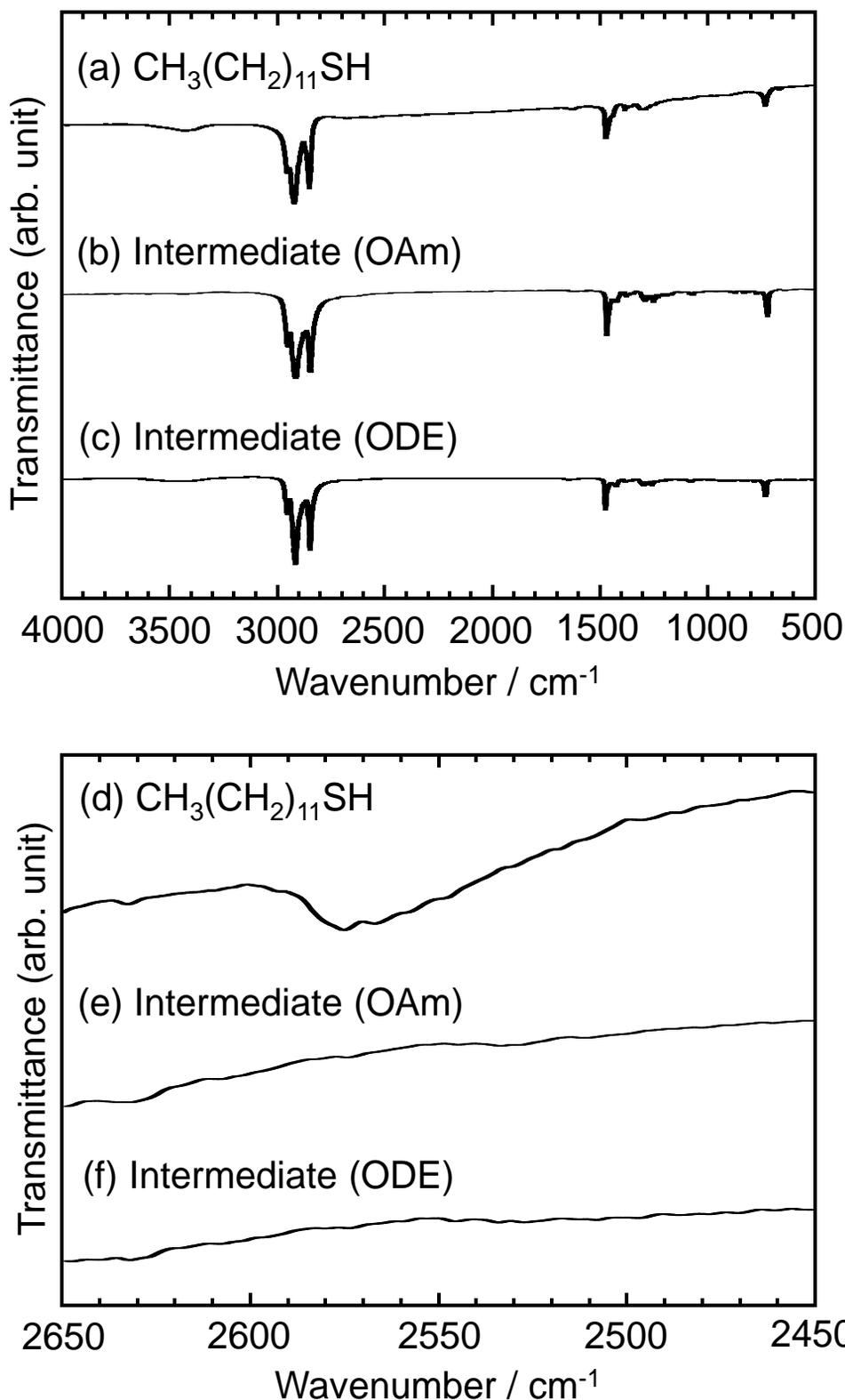
Fig. 4 (a-c) FT-IR spectra of (a) 1-dodecanethiol and (b,c) intermediate prepared by heating at 180 °C in (b) OAm or (c) ODE. (d-f) show the enlarged spectra between 2650 and 2450 cm<sup>-1</sup> for the (a-c) samples.
