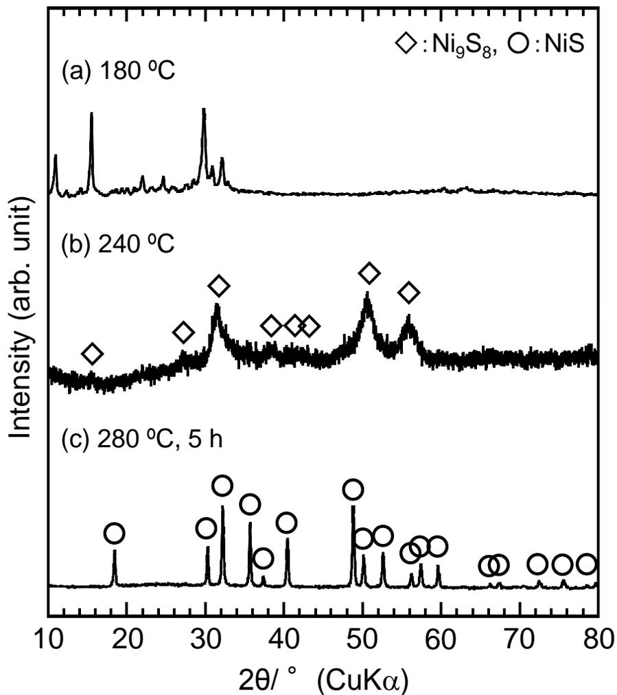
Fig. 2 XRD patterns of the samples prepared by heating at (a) 180 °C, (b) 240 °C, and (c) 280 °C for 5 h in octadecene (ODE).
