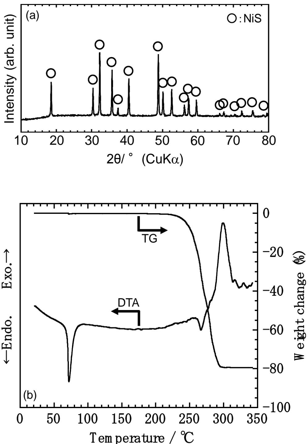
Fig. 3 (a) XRD pattern of the sample prepared by heating the intermediate in ODE at 280 °C for 5 h (“Route 1” shown in Scheme 1). (b) DTA-TG curves of the intermediate under N<sub>2</sub> flow.
