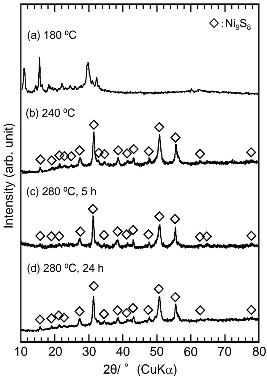
Fig. 1 XRD patterns of the samples prepared by heating at (a) 180 °C, (b) 240 °C, (c) 280 °C for 5 h, and (d) 280 °C for 24 h in oleylamine (OAm).
