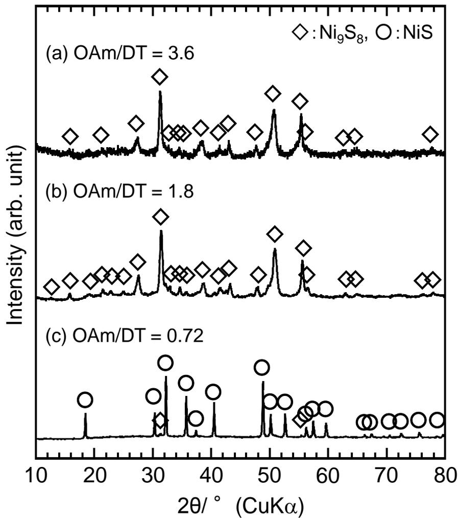
Fig. 6 XRD patterns of the samples prepared by changing the amount of OAm ("Route 3" shown in Scheme 1).
