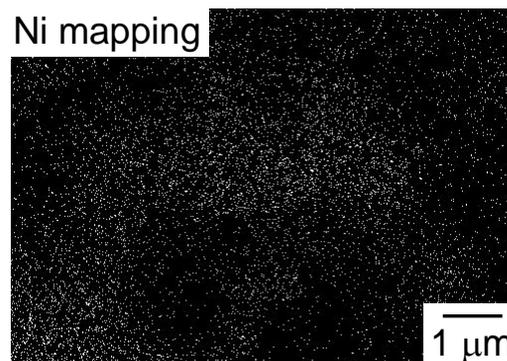
Fig. 7 SEM images and EDX mapping images for Ni element of (a) the composite electrode prepared by wet milling of NiS, solid electrolyte, and VGCF in hexane, and (b) the composite electrode prepared by hand-grinding of NiS, solid electrolyte, and VGCF in a mortar.
