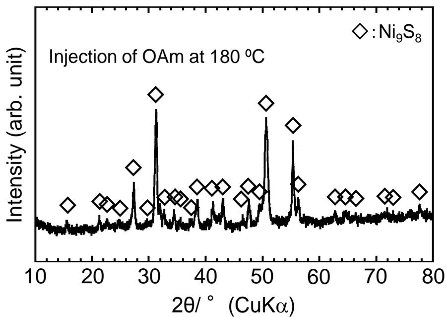
Fig. 5 XRD pattern of the sample prepared by injection of OAm at 180 °C (“Route 2” shown in Scheme 1).
