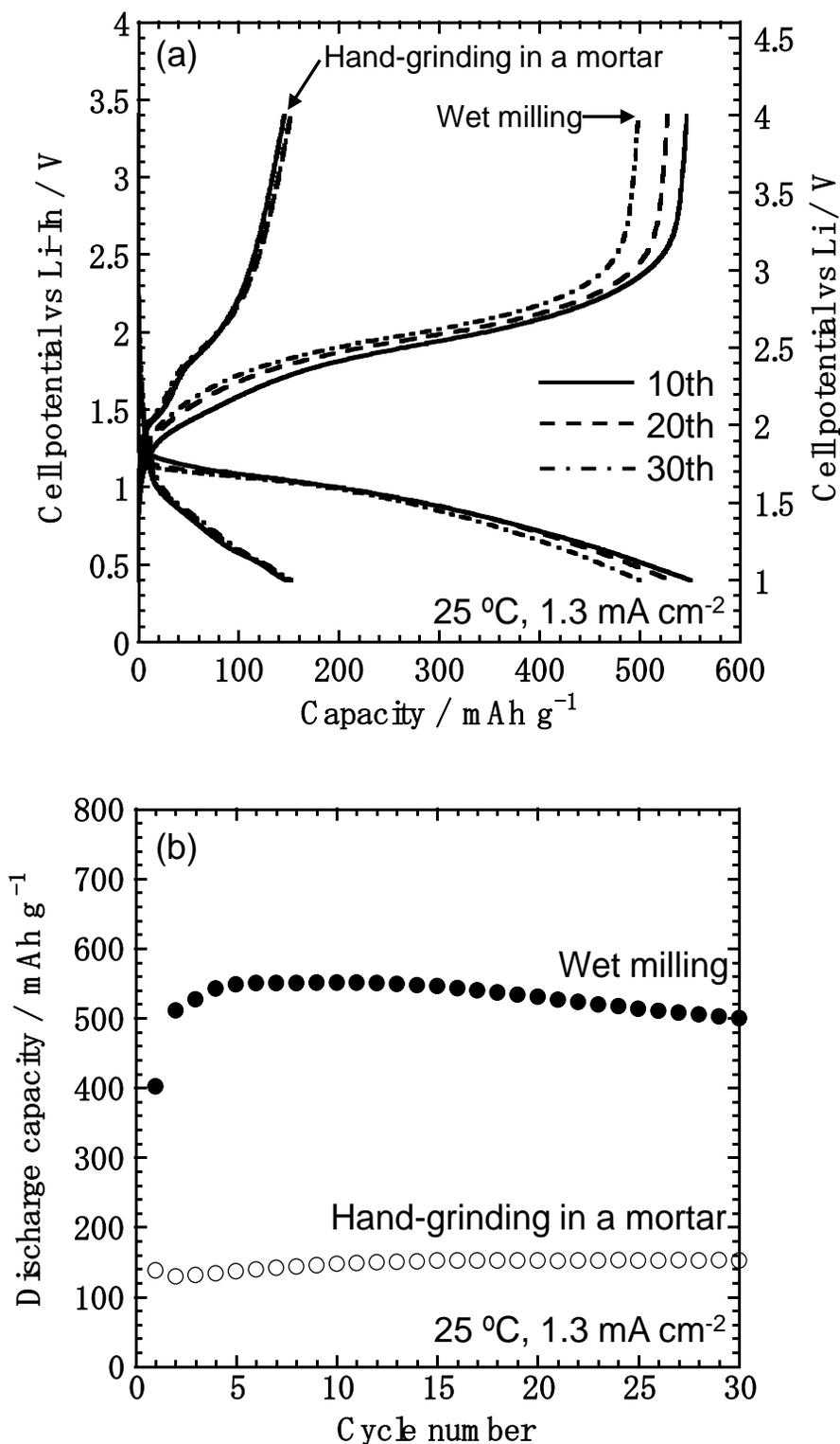
Fig. 8 (a) Charge-discharge curves and (b) cycle performance of the all-solid-state cells with the composite electrode prepared by wet milling in hexane and by hand-grinding in a mortar under the current density of 1.3 mA cm<sup>-2</sup>.
