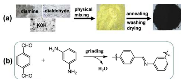
Fig. 1 (a) Schematic illustration of preparing MPCs from diamine and dialdehyde, and (b) reaction equation showing the condensation between terephthalaldehyde and m -phenylenediamine to form imine-based polymer with water as only by-product.
