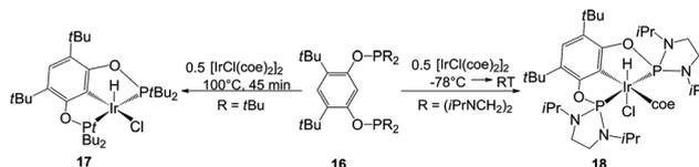
Scheme 8 Synthesis of the iridium P(III) analogues of complex **14**, for comparison in the catalytic C–H borylation of arenes.
