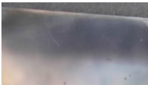
Figure 6 Photograph showing the gradient deposition viewed from transmitted (top) and reflected light from an auric acid and butyltin trichloride ratio of 0.06 on the top plate.
