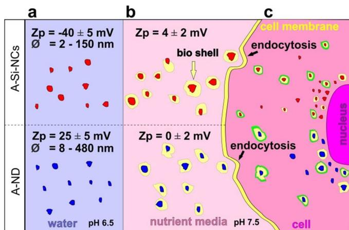
**Fig. 7** Schematic representation of nanoparticles behavior in various solvents and their changes of  $\zeta$  (zeta – potential) (a) nanoparticles in water ( $\emptyset$  – diameter of particle), (b) nanoparticles in nutrient media covered with bio-molecular shell (possibly protein corona) which changes the overall zeta-potential (c) nanoparticles in the cell tend to agglomerate in close proximity of nucleus, the presumed way of entering the cell is endocytosis.
