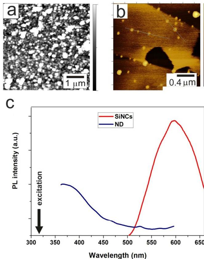
**Fig. 1** Characterization of Si-NC and ND nanoparticles, AFM image of (a) A-NDs (Z scale 50 nm) and (b) A-Si-NCs (Z scale 15.5 nm) on highly ordered pyrolytic graphite, (c) PL spectra of A-Si-NCs (intensity divided by 10) and A-NDs in ethanol (excited at 320 nm, measured with the FluoroMax-3 spectrometer, corrected for sensitivity of the apparatus and Raman scattering of solvent).
