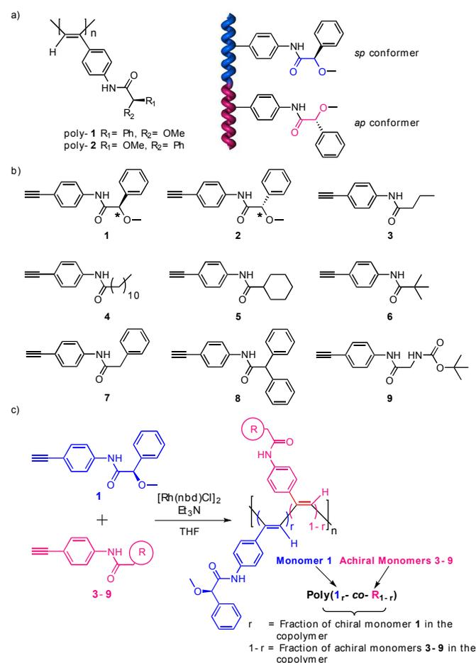
**Figure 2.** Structures of homopolymers, monomers and copolymer synthesis. a) Structures of poly-**1**, poly-**2** and *sp/ap* conformations. b) Structures of monomers **1-9**. c) Synthesis, structures and notation of copolymers.
