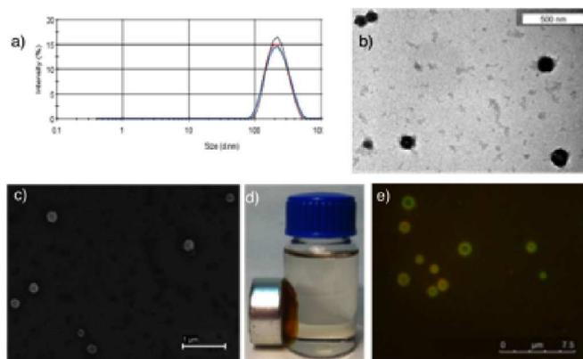
**Figure 5.** Copolymer nanospheres and encapsulating properties. a) DLS trace. b) TEM image of copolymer- $\text{Ba}^{2+}$  metal complex nanospheres. c) SEM images of the nanospheres. d) Vial showing the nanospheres encapsulating iron oxide magnetic nanoparticles placed close to a magnet. e) Confocal images of the nanospheres encapsulating rhodamine B.
