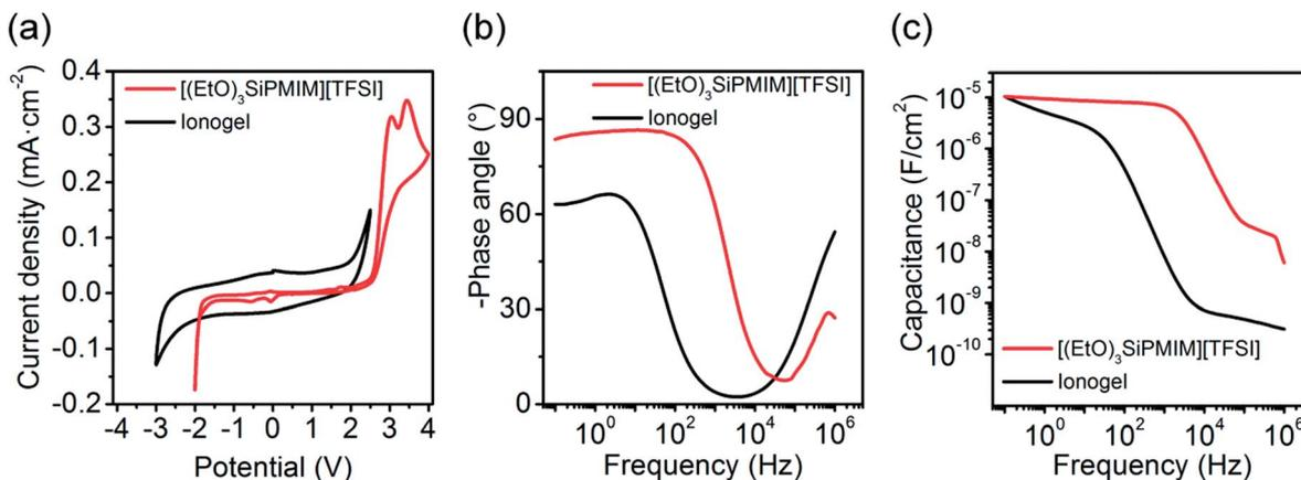
Fig. 4 (a) Cyclic voltammograms of [(EtO)<sub>3</sub>SiPMIM][TFSI] and spray-coated ionogels. Frequency dependent phase angle (b) and calculated specific capacitance (c) of the ionic liquid and ionogel (measured in ambient air).
