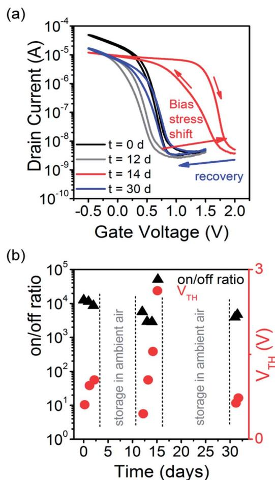
Fig. 6 (a) Transfer characteristics ( $V_{\text{D}} = -1.0 \text{ V}$ ) of the ionogel-gated P3HT transistor after 0, 12, 14 and 30 days of measurements and storage in ambient air (voltage sweep rate  $80 \text{ mV s}^{-1}$ ). (b) Extracted on-off ratios and threshold-voltages for this device after bias stress and storage in air.
