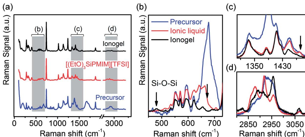
Fig. 2 Raman spectra of the pure [(EtO)<sub>3</sub>SiPMIM][TFSI] ionic liquid, the final ionogel and the precursor solution between (a) 150 and 3100 cm<sup>-1</sup>, (b) 450 and 710 cm<sup>-1</sup>, (c) 1300 and 1500 cm<sup>-1</sup>, and (d) 2800 and 3100 cm<sup>-1</sup>.
