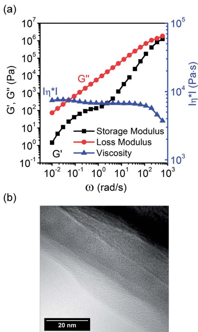
Fig. 3 (a) Loss ( $G''$ ) modulus, storage ( $G'$ ) modulus and viscosity ( $|\eta^*|$ ) versus angular frequency ( $\omega$ ) in the viscoelastic regime for a silane-based ionogel. (b) HRTEM image of the spray-coated ionogel on a thin carbon membrane.
