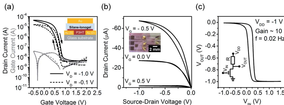
Fig. 5 Transfer characteristics of the ionogel-gated P3HT transistor (sweep rate 80 mV s<sup>-1</sup>); inset: device geometry (S – source, D – drain). (b) Output characteristics, inset: optical image of the device with evaporated gold gate electrodes. (c) Transfer curve of the resistor-loaded inverter with the ionogel-gated P3HT transistor, inset: circuit diagram.
