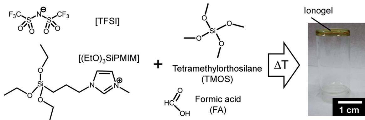
Fig. 1 Molecular structures of the ionic liquid [(EtO)<sub>3</sub>SiPMIM][TFSI] and network precursors with optical image of the resulting ionogel.
