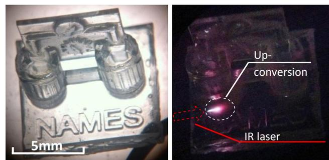
**Fig. 7.** Photograph of a 3D-printed model shaped as a photoelectrochemical (PEC) cell using these new RE-doped up-conversion organic resins. NAMES logo stands for our research group, nanomaterials and spectroscopy, www.names-ull.es.
