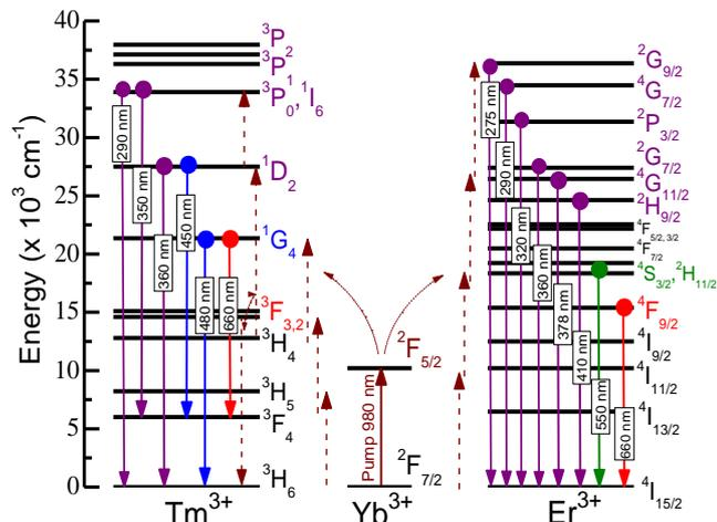
**Fig. 2.** Energy level diagram of  $\text{Yb}^{3+}$ ,  $\text{Tm}^{3+}$  and  $\text{Er}^{3+}$  ions. Up-conversion mechanisms, pumping and main emission transitions are arrowed and labelled with corresponding wavelengths.
