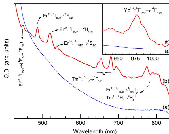
**Fig. 1.** Absorption spectra of (a) an undoped and (b) a RE-doped ( $\text{Yb}^{3+}:\text{Er}^{3+}:\text{Tm}^{3+}$ ) organic resin, in some parts of the visible and NIR range, where the large cross-section of  $\text{Yb}^{3+}$  ions (inset) act as infrared collecting antenna.
