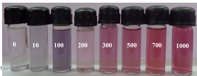
Fig.4: Colour developed by the addition of mercury ion (0-1000 nM) into Au + colourless aqueous solution
