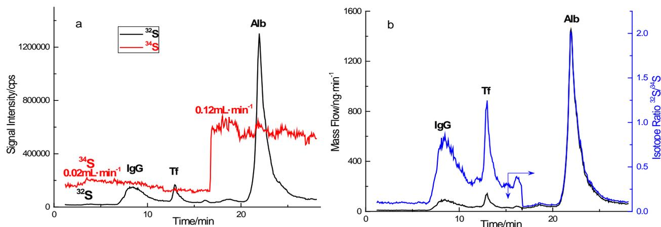
Fig 6 Mass spectrum of human serum, a: HPLC-ID-ICP-MS; b: chromatogram of mass flow of sulfur and isotope ratio
