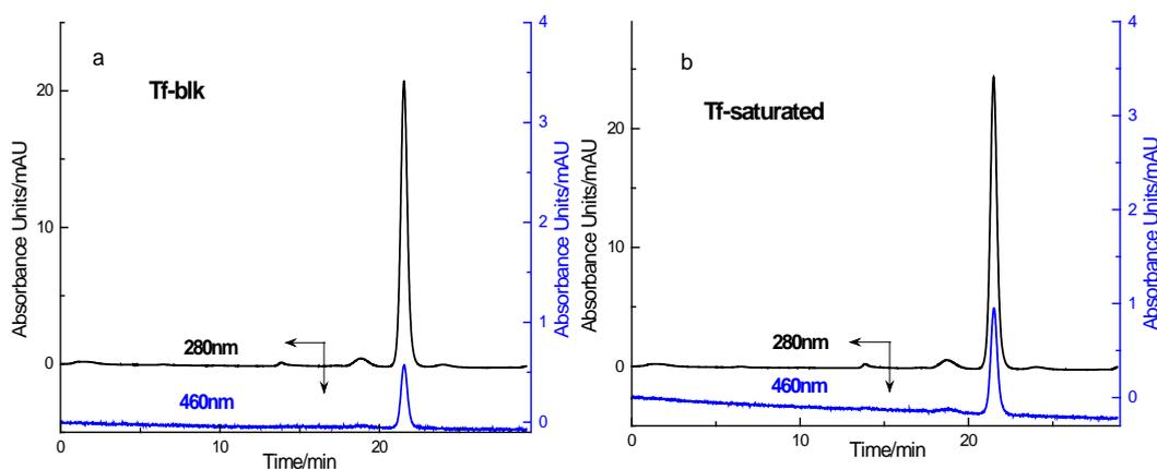
Fig. 3 Liquid chromatography of Tf blk (a) and Tf with saturation (b) using UV detection of HPLC at 280nm and 460nm
