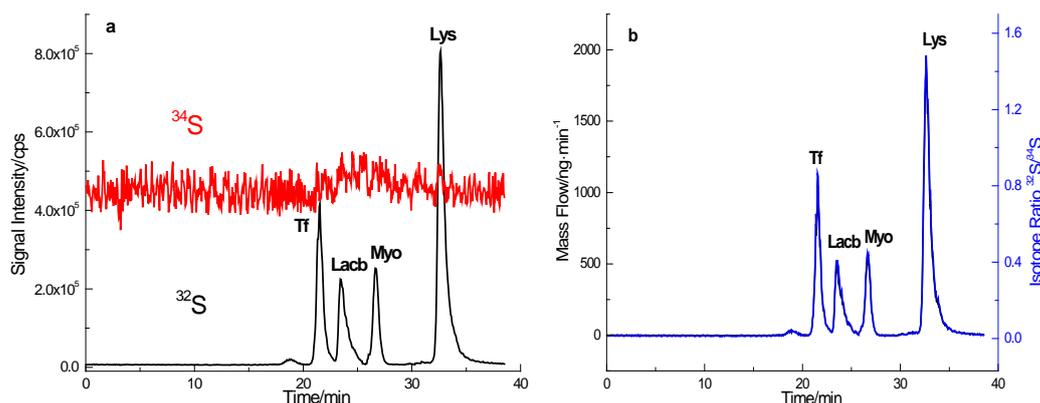
Fig. 2 Mass spectrum of mixed standard proteins, a: HPLC-ID-ICP-MS; b: chromatogram of mass flow of sulfur and isotope ratio
