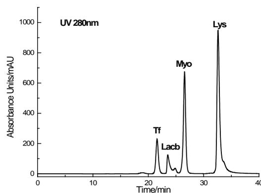
Fig. 1 Liquid chromatography of four standard proteins
