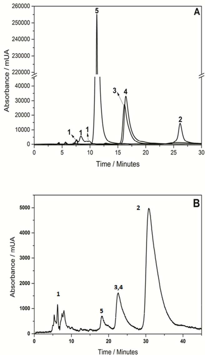
**Figure 2.** HPLC/DAD chromatograms obtained for 20  $\mu\text{L}$  (A) of standard solution of  $8 \times 10^{-5} \text{ mol L}^{-1}$  of the hair dyes: (1) BB99, (2) AV43, (3) BB16, (4) BR76 and (5) BY57, respectively and their mixture (B). Mobile phase: ACN/phosphate buffer ( 45:55, v/v ). T: 40°C, flow-rate: 1.0 mL  $\text{min}^{-1}$ ; C18 phase. Wavelength of standard dyes:  $\lambda = 383 \text{ nm}$ ; 482 nm; 499 nm; 523 nm e 618 nm. Wavelength of mixture:  $\lambda = 413 \text{ nm}$ .
