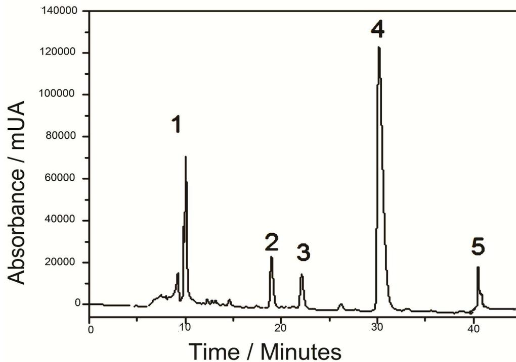
**Figure 5.** HPLC/DAD chromatograms obtained for a commercial hair dye sample assigned as HF 65 (Arianor, LCW Dyes, São Paulo, Brazil). ACN/ H<sub>2</sub>O + 40 mM BMIm[NTf<sub>2</sub>] 35:65 (v/v). T: 40 °C, flow-rate: 0.4 mL min<sup>-1</sup>; C18 column.  $\lambda$ = 413 nm. 1: BB99, 2: AV43, 3: BB16, 4: BR76 and 5: BY57.
