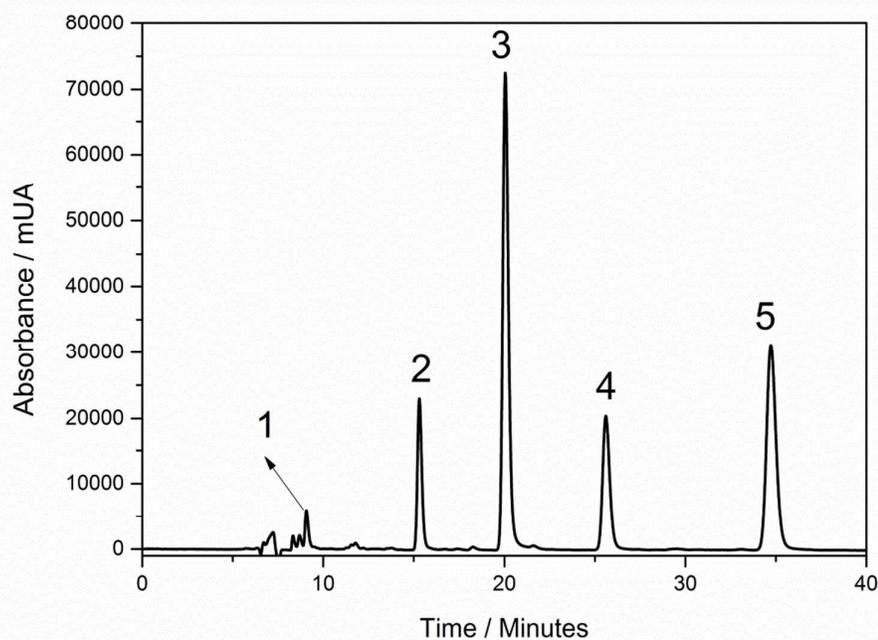
**Figure 4.** HPLC/DAD chromatogram obtained for the mixture of 1: BB99, 2: AV43, 3: BB16, 4: BR76 and 5: BY57 dyes at concentration of  $8 \times 10^{-5} \text{ mol L}^{-1}$ , extracted in 50:50 ACN/H<sub>2</sub>O and eluted with ACN/ H<sub>2</sub>O + 40 mM BMIm[NTf<sub>2</sub>] 35:65 (v/v). T: 40°C, flow-rate: 0.4 mL min<sup>-1</sup>; C18 column.  $\lambda = 413 \text{ nm}$ .
