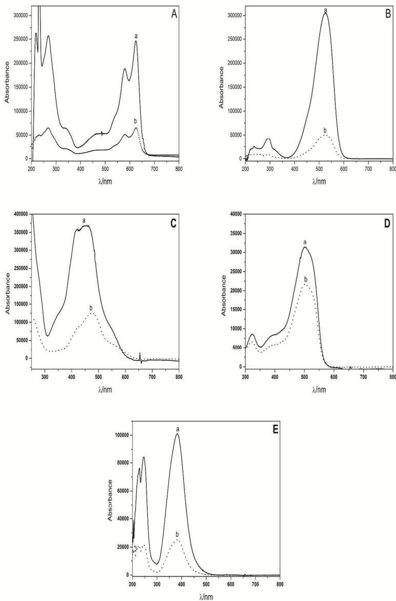
**Figure 6.** (a) UV-Vis spectra obtained from hydrodynamic chromatograms corresponding to each retention time of (A): BB99, (B): AV43, (C): BB16, (D): BR76 and (E): BY57, respectively for standard dye sample (a) and commercial sample (b).
