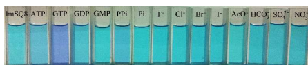
Fig. 1 Color changes of ImSQ8 (10 \mu\text{M} ) upon addition of sodium salt of various anions (1.0 equiv) in HEPES buffer (10 mM, pH = 7.2).
